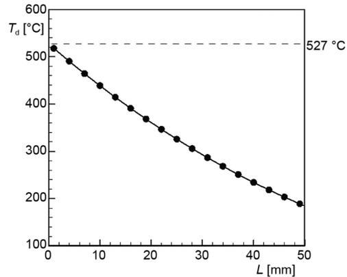
Figure 7. The apparent temperature vs. the width of the vibrating screen
