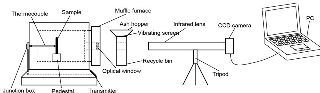
Figure 2. The schematic of experimental rig
