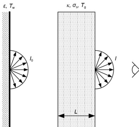
**Figure 6.** Schematic of the infrared temperature measurement for 1-D plane-parallel slab model
