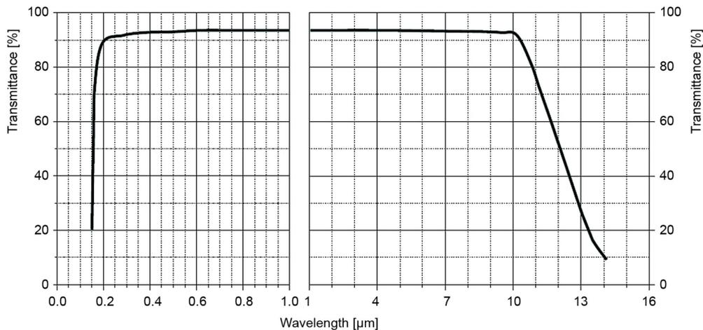
Figure 3. The transmittance curve of BaF
