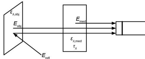
Figure 1. The schematic of the effective radiation in infrared temperature measurement
