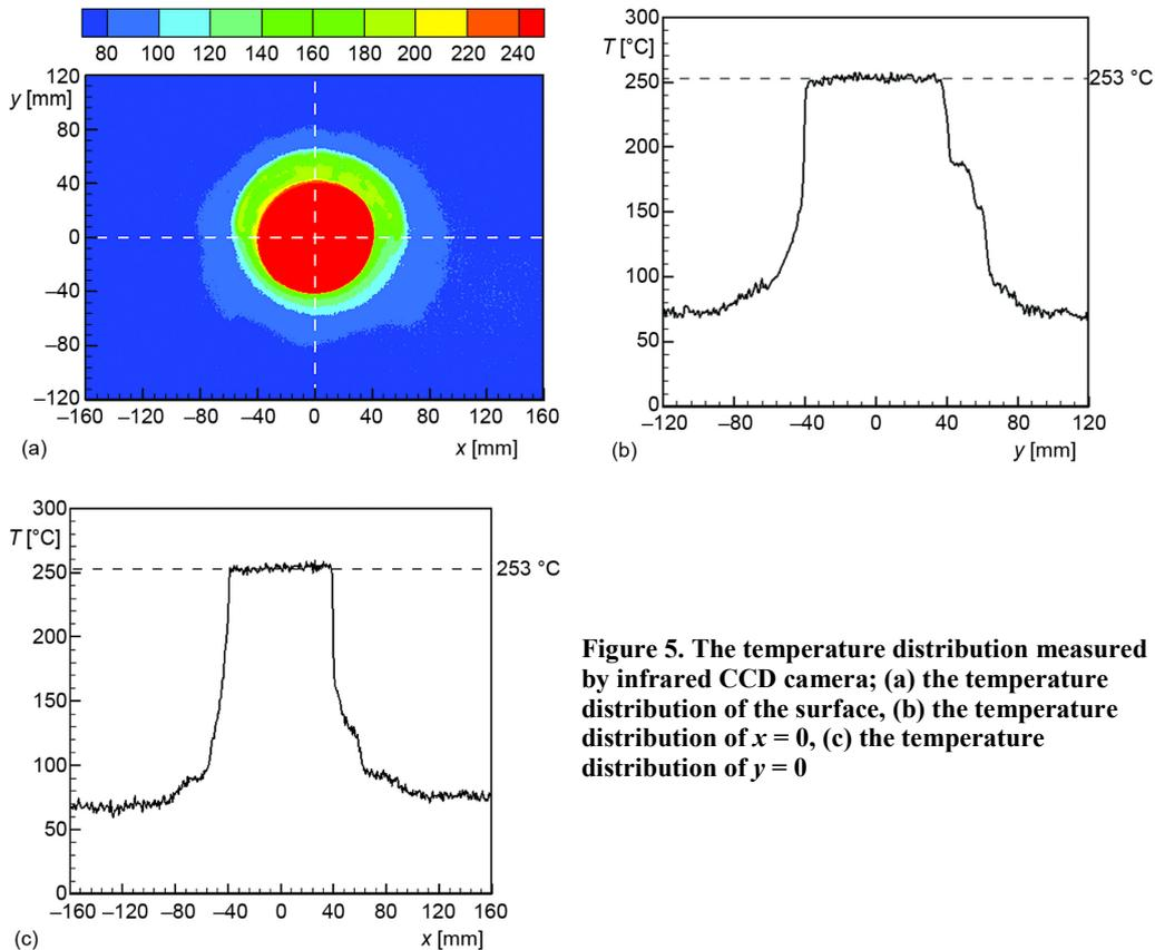
**Figure 5.** The temperature distribution measured by infrared CCD camera; (a) the temperature distribution of the surface, (b) the temperature distribution of  $x = 0$ , (c) the temperature distribution of  $y = 0$
