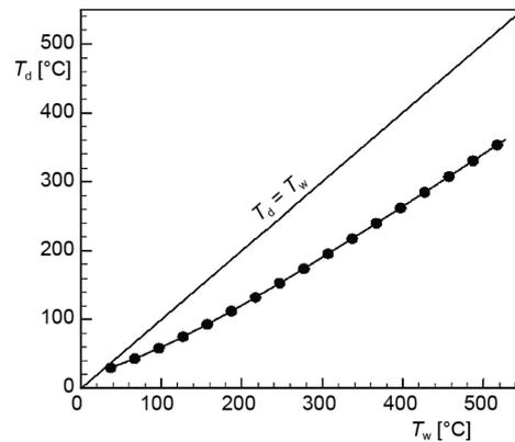
Figure 8. The apparent temperature vs. the set temperature of the muffle furnace
