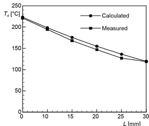
Figure 9. Comparison of the calculated and measured temperatures at different widths of the vibrating screen
