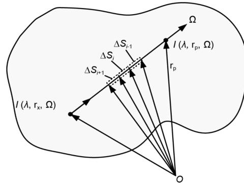
Figure 4. The schematic of arbitrary directional radiative intensity computation
