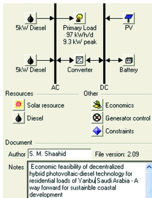
Figure 4. Schematic of hybrid PV-diesel-battery power system
