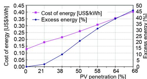
**Figure 6. Impact of PV penetration on COE and excess energy generated at Yanbu for hybrid system**
