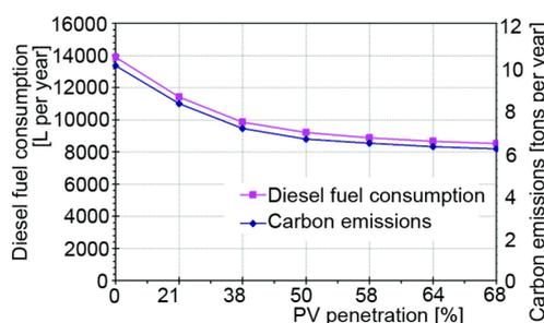
**Figure 5. Impact of PV penetration on diesel consumption and carbon emissions at Yanbu for hybrid system**
