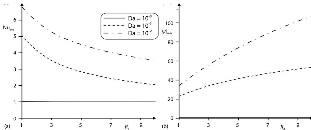
Figure 5. Variation of the average Nusselt number (a) and maximum absolute value of the stream function (b) with radiation parameter and Darcy number for  $C = 3$
