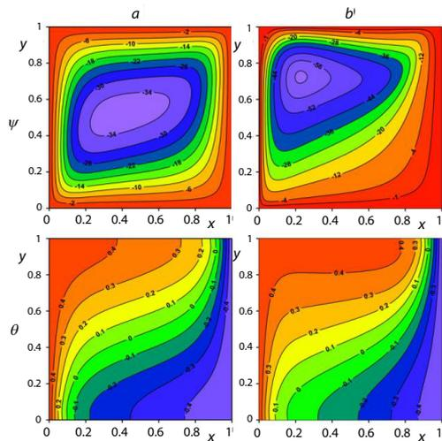
Figure 4. Streamlines  $\psi$  and isotherms  $\theta$  at  $Da = 10^{-3}$ ,  $R_d = 5$ ; (a)  $C = 1$ , (b)  $C = 6$
