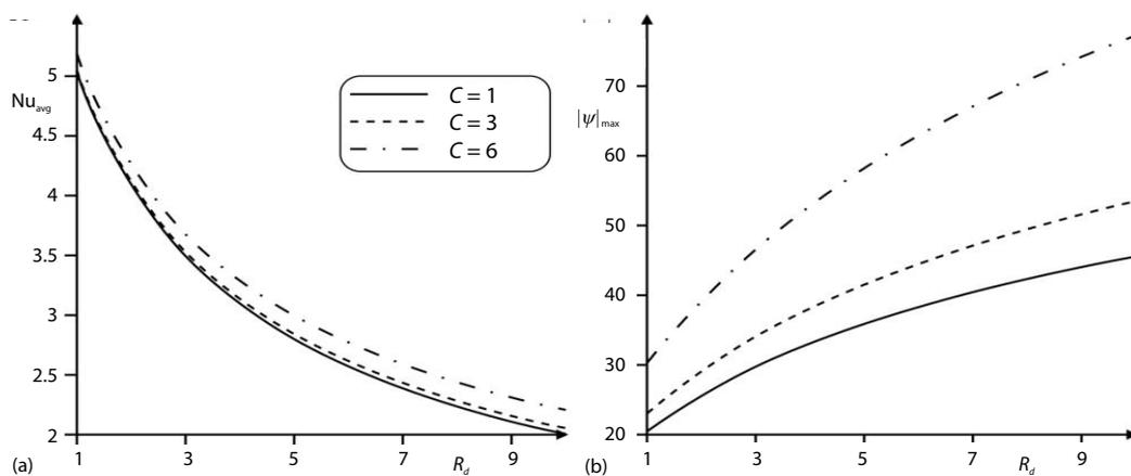
Figure 6. Variation of the average Nusselt number (a) and maximum absolute value of the stream function (b) with radiation parameter and viscosity variation parameter for  $Da = 10^{-3}$
