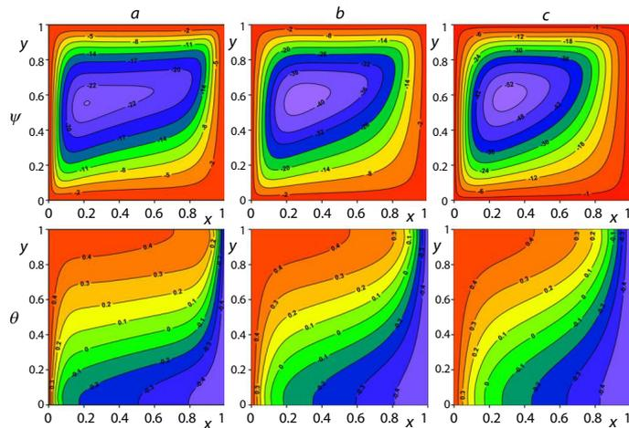
Figure 2. Streamlines  $\psi$  and isotherms  $\theta$  at  $Da = 10^{-3}$ ,  $C = 3$ ; (a)  $R_d = 1$ , (b)  $R_d = 5$ , (c)  $R_d = 10$
