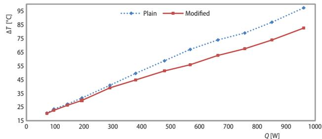
Figure 5. The overall temperature difference for both layouts at various heat inputs
