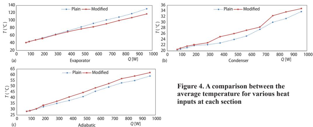
**Figure 4. A comparison between the average temperature for various heat inputs at each section**
