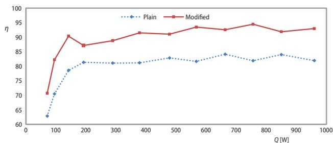
Figure 6. The thermal efficiency of both layouts at various heat inputs
