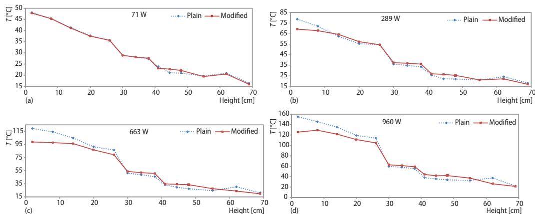
Figure 2. The TPCT temperature profiles at various heat inputs
