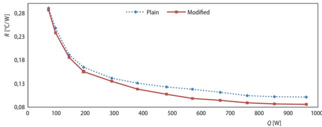
**Figure 3. A comparison between the TPCT overall thermal resistance at various heat inputs**
