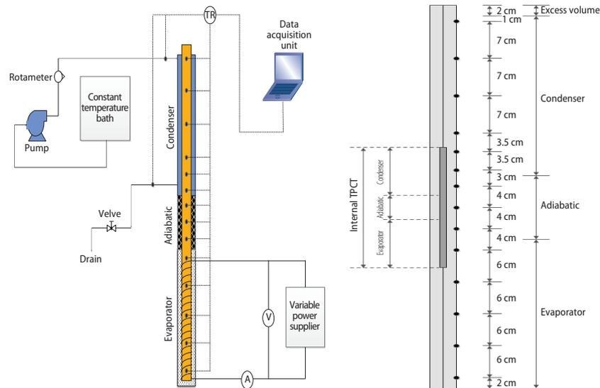
**Figure 1. (a) A schematic of the experimental rig and (b) position of internal TPCT and thermocouples**
