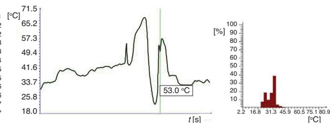
**Figure 2. Development of surface temperatures and temperature histogram on the head (max.  $\theta_{si} = 67.1$  °C) and Al plate ( $\theta_{si} = 53$  °C) along the line L1 shown in fig. 1**
