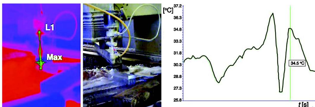
Figure 4. View of cutting Al plate + stainless steel in a sandwich configuration and evaluation of its IR method at the beginning of operation and development of temperatures
