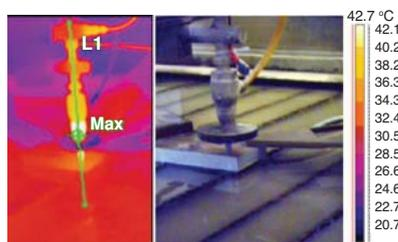
**Figure 1. View of cutting Al plate of thickness 20 mm and its IR evaluation method before the end of the cutting operation – 4<sup>th</sup> cut**
