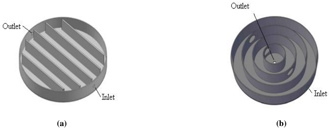
Figure 1. Schematic of receiver flow path configurations (a) Straight path (b) Spiral path
