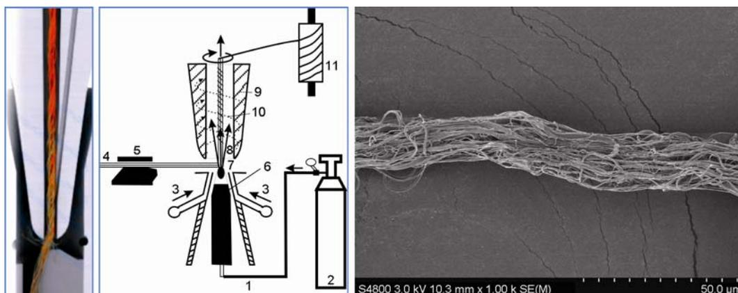
**Figure 2. Set-up of fascinated nanofiber yarns' fabrication (Patent No. ZL 2013 2 0720637.9) and nanofiber yarns; 1 – tube, 2 – gas storage, 3 – hot air, 4 – yarn, 5 – yarn guide, 6 – solution, 7 – bubble, 8 – nanofiber, 9 – nozzle, 10 – vortex, 11 – wind-up**
