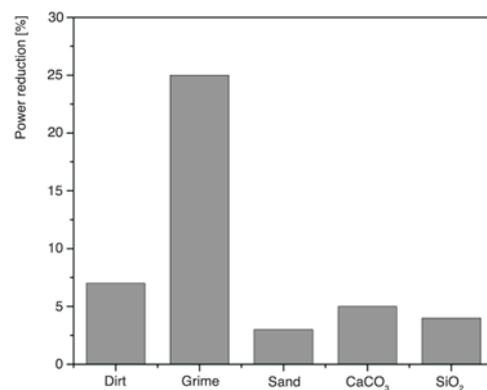
**Figure 4. Influence of different particles on solar cells power reduction**
