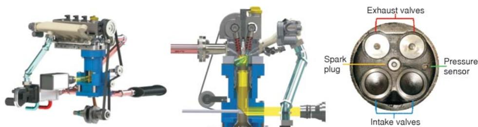
**Figure 1. Schematic of the experimental set-up and bottom field of view of the combustion chamber**
