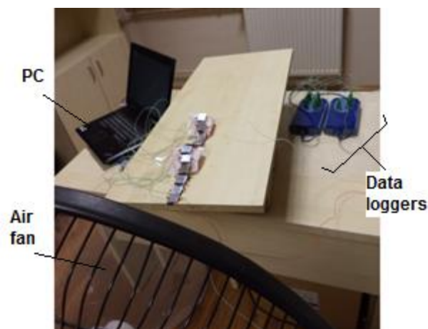
Fig. 3. Experimental setup in the assessment of the experimental convective heat transfer coefficients on the conductive surfaces. Centered is the arbitrary-shape body.
