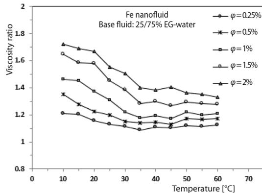
**Figure 3.** The viscosity ratio of Fe nanoparticles in (25/75 wt.%) EG-water mixture vs. temperature at different volume concentrations
