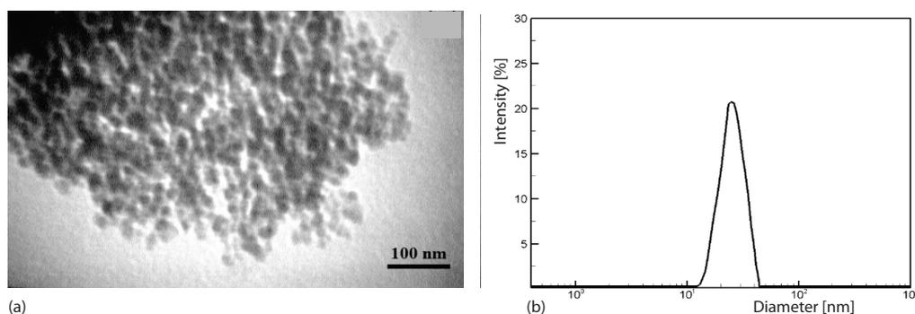
Figure 1. (a) TEM image of nanoparticles, (b) diameter distribution of nanoparticles obtained by dynamic light scattering
