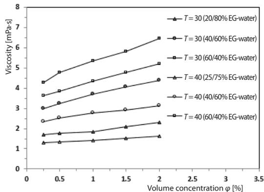
**Figure 4.** The viscosity of Fe nanoparticles in different base fluids vs. volume concentration at  $T = 30$  and  $40$  °C
