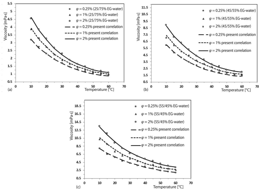
**Figure 7.** Comparison of the experimental viscosity of Fe nanoparticles in a mixture of EG-water with the presented correlation at three different volume concentrations of 0.25, 1, and 2%
