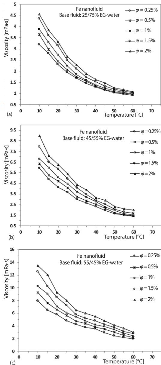
**Figure 2. Viscosity of Fe nanoparticles in (a) 25/75%, (b) 45/55%, and (c) 55/45% EG-water *vs.* temperature at different volume concentrations**
