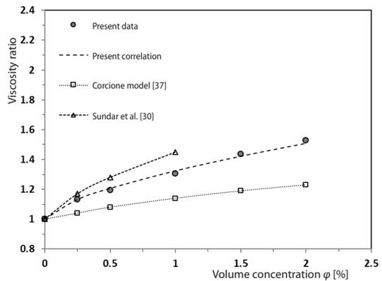
**Figure 6. Comparison between the viscosity ratios of Fe nanoparticles in a mixture of EG-water (25/75 wt.%) and the predicted values from current correlation and previous models ( $T = 30$  °C)**
