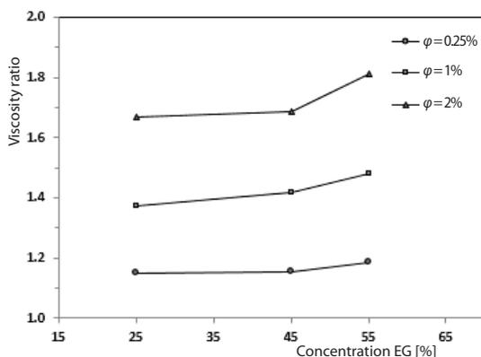
**Figure 5.** The viscosity ratio of Fe nanofluids vs. concentration of EG mixed with water at  $\phi = 0.25, 1,$  and  $2\%$
