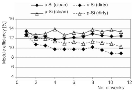
**Figure 9.** Variation of weekly average module efficiency of c-Si and p-Si modules at 9 a. m.
