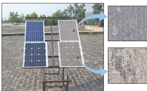
Figure 1. The PV modules used in the study with dust deposited on dirty modules surfaces after 11 weeks
