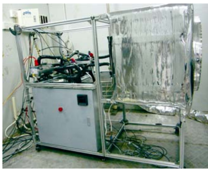
Figure 2. The experimental platform of gas-mixing HPACS for PEV
