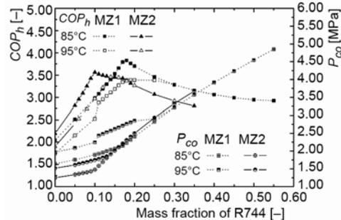
Figure 5.  $COP_h$  and  $P_c$  vs. mass fraction of R744 for different outlet water temperature
