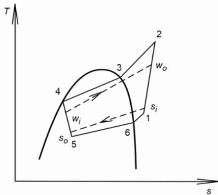
Figure 1. Schematic of subcritical heat pump using MZ1 or MZ2 as refrigerant
