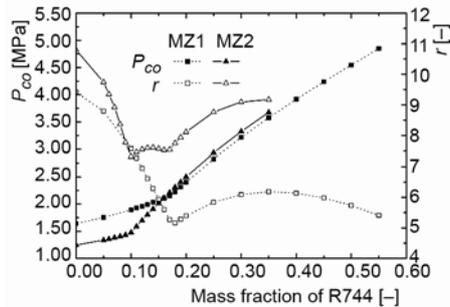
Figure 4. Condensation pressure and compression ratio vs. mass fraction of R744
