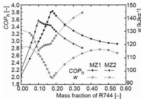
**Figure 2. *COP<sub>h</sub>* and compressor power of MZ1 and MZ2 vs. mass fraction of R744**
