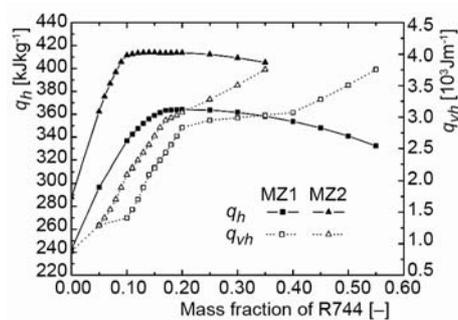
**Figure 3. *q<sub>h</sub>* and volumetric heating capacity of MZ1 and MZ2 vs. mass fraction of R744**
