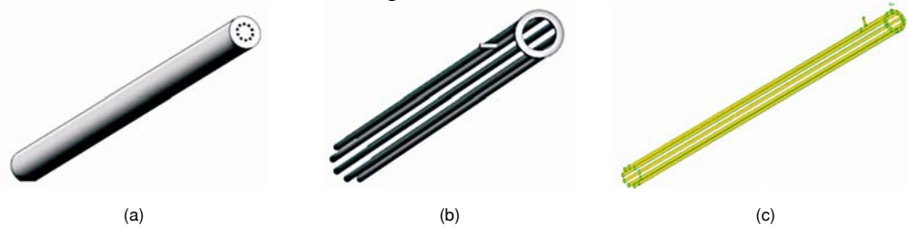
Figure 2. The 3-D model, the domain field, and the mesh of ventilation rate standard bar
