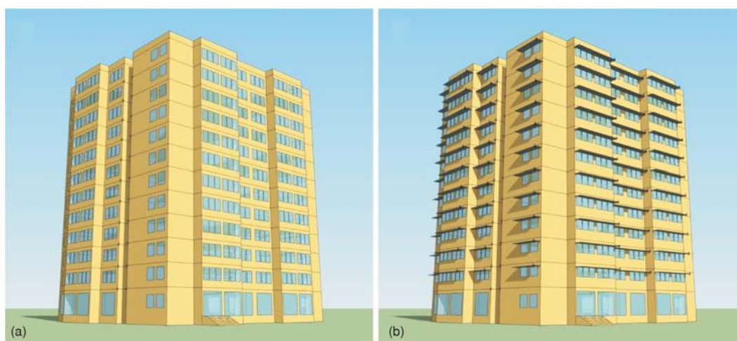
Figure 3. Overview of the dormitory with “base” and “optimal” façade design with shading devices upgrading in terms of energy saving
