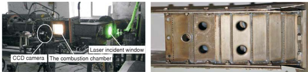
Figure 2. Experiment system and the double swirl annular combustor geometry
