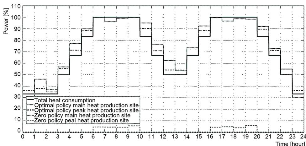
Figure 2. Heat production with fixed and optimized supply temperatures
