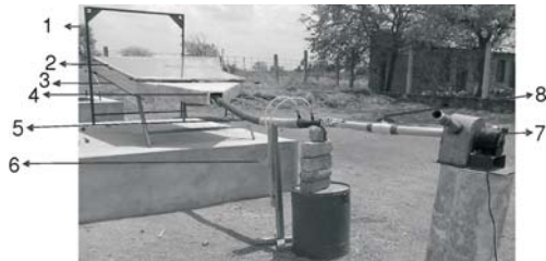
Figure 1. Set-up of double pass SAH, with vertically arranged wire mesh 1 – adjustable vertical stand, 2 – glass cover, 3 – insulation, 4 – air inlet, 5 – air outlet, 6 – U tube manometer, 7 – blower, 8 – control valve
