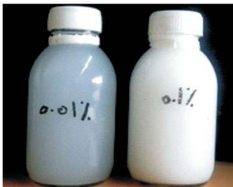
**Figure 3. The nanofluids used during the tests**
