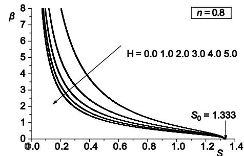
**Figure 3.** Variations of film thickness with the unsteadiness parameter at selected values of Hartmann number
