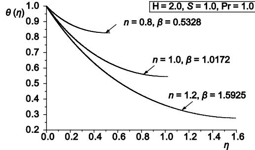
Figure 7. Effects of the power law index on the temperature profiles
