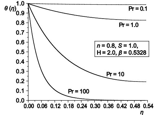
Figure 9. Effects of the Pr on the temperature profiles
