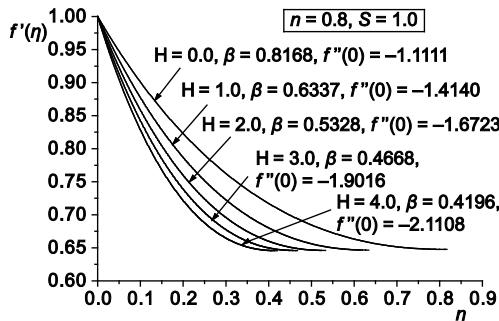
**Figure 4.** Effects of the Hartmann number on the velocity profiles
