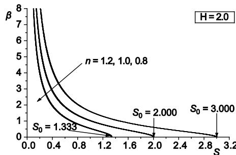
**Figure 2.** Variations of film thickness with the unsteadiness parameter at selected values of  $n$
