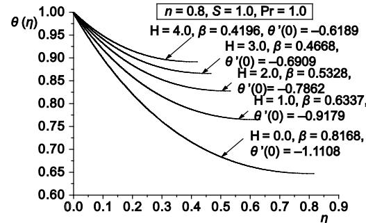
**Figure 5.** Effects of the Hartmann number on the temperature profiles
