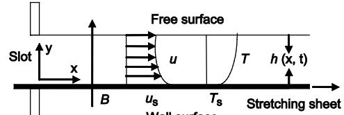
Figure 1. Schematic of the physical system
