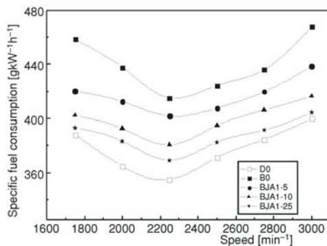
Figure 4. The specific fuel consumption vs. engine speed
