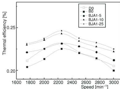
Figure 6. The thermal efficiency versus engine speed
