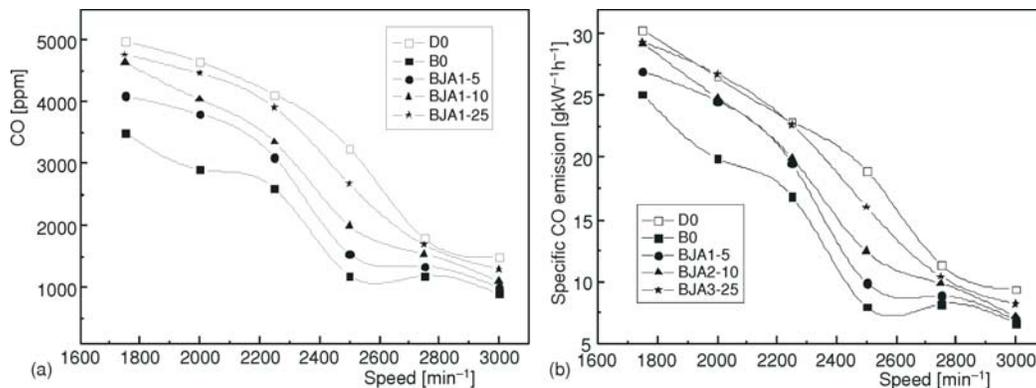
Figure 9. CO emission vs. engine speed (a) in ppm, (b) in g/kWh
