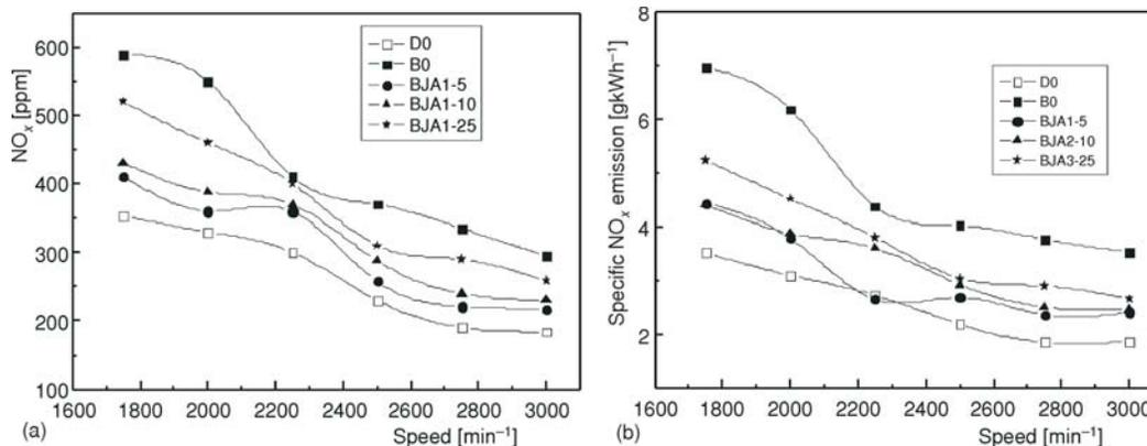
Figure 7.  $\text{NO}_x$  emission vs. engine speed (a) in ppm, (b) in g/kWh
