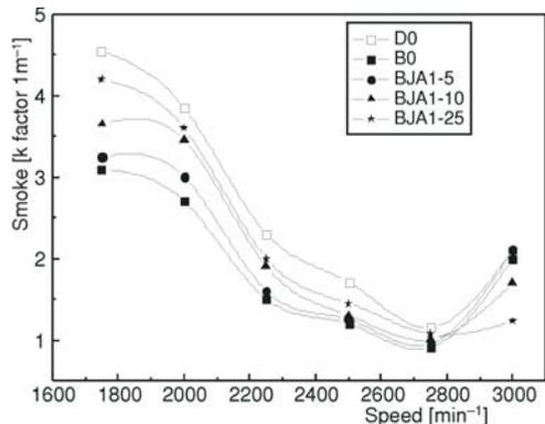
Figure 8. Smoke emission vs. engine speed
