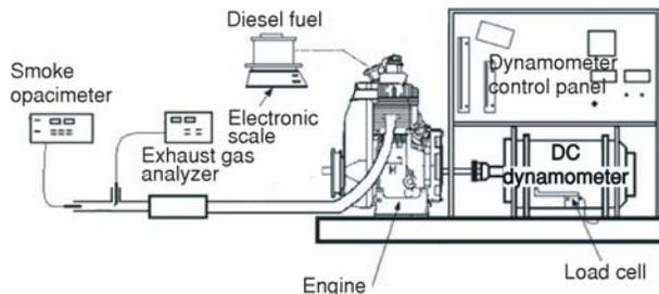
**Figure 1. Schematic representation of the experimental apparatus**
