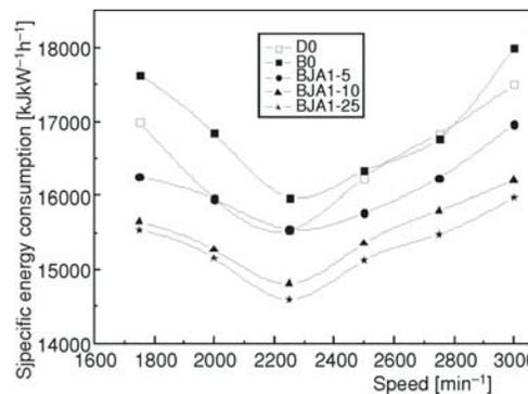
Figure 5. The specific energy consumption vs. engine speed
