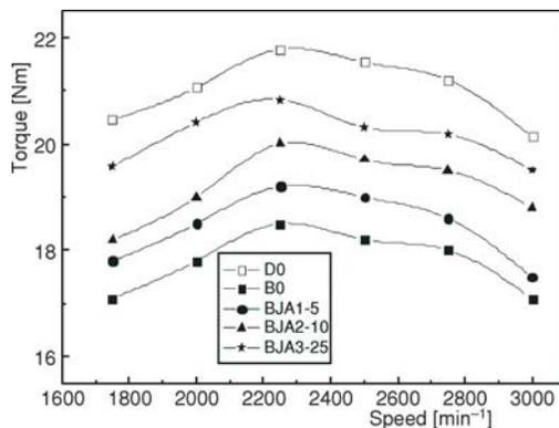
**Figure 2. The brake torque vs. engine speed**
