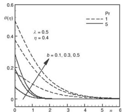
Figure 4. Effects of Prandtl number and convection-conduction parameter  $b$  on temperature profiles
