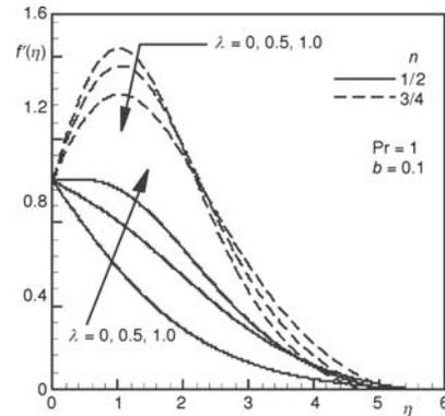
Figure 2. Effects of index parameter  $n$  and buoyancy parameter  $\lambda$  on velocity profiles
