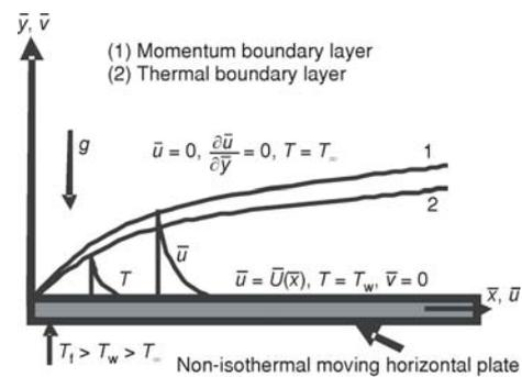
Figure 1. Schematic representation of the boundary layer flow of a continuously moving plate
