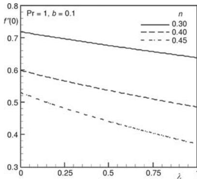
Figure 5. Variation of friction factor vs. buoyancy parameter  $\lambda$  for different  $n$
