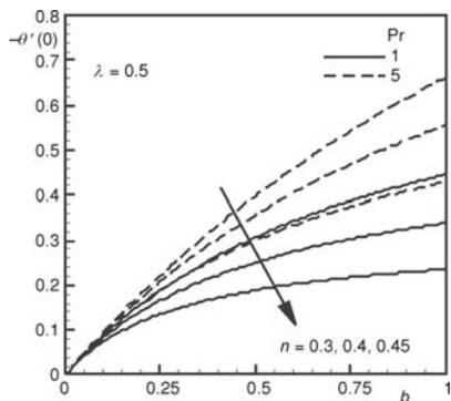
Figure 7. Variation of dimensionless heat transfer rates vs. convection-conduction parameter  $b$  for different Prandtl number  $Pr$
