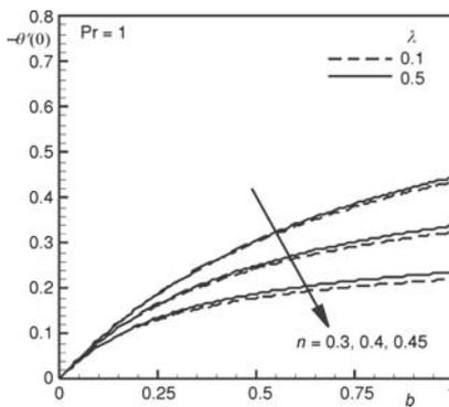
Figure 6. Variation of dimensionless heat transfer rates vs. convection-conduction parameter  $b$  for different buoyancy parameter  $\lambda$
