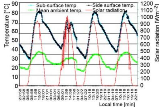
**Figure 6.** The sub- and side-surface temperature curve of the paraffin wax in the cooker with a reflector angle of 60° and the solar radiation intensity for the region on July 3-6, 2011 (for color image see journal web-site)
