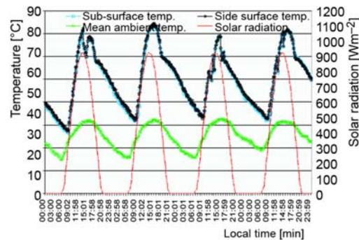
**Figure 7.** The sub- and side-surface temperature curve of the paraffin wax in the cooker with a reflector angle of 45° and the solar radiation intensity for the region on July 8-11, 2011
