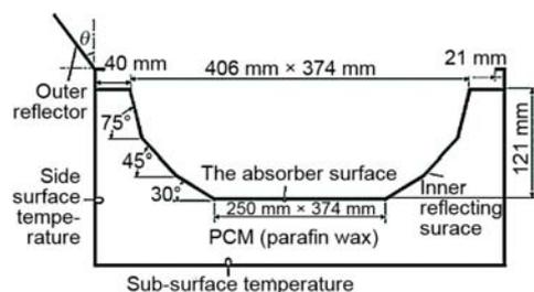
**Figure 1.** Schematic diagram of the box-type solar cooker with inner and outer reflectors
