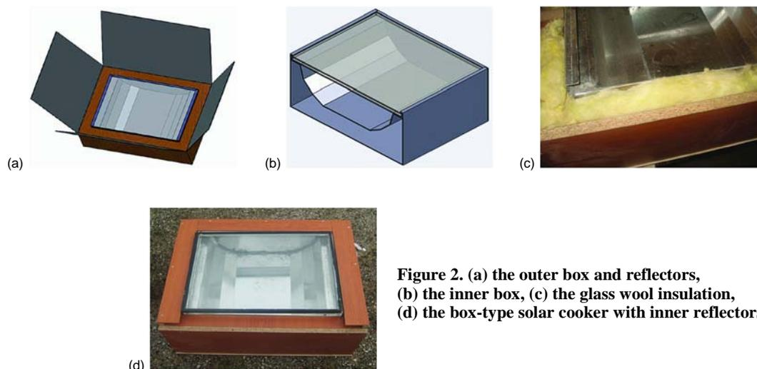
**Figure 2. (a) the outer box and reflectors, (b) the inner box, (c) the glass wool insulation, (d) the box-type solar cooker with inner reflectors**
