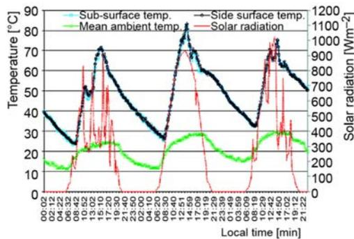
**Figure 5.** The sub- and side-surface temperature curve of the paraffin wax in the cooker with a reflector angle of 30° and the solar radiation intensity for the region on June 29-July 1, 2011 (for color image see journal web-site)
