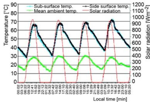
**Figure 4. The sub- and side-surface temperature curve of the paraffin wax in the cooker with insulation and the solar radiation intensity for the region on June 22-26, 2011**
