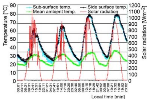
**Figure 3. The sub- and side-surface temperature curve of the paraffin wax in the cooker without insulation and the solar radiation intensity for the region on June 17-20, 2011**
