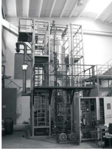
Figure 9. Pilot FICFB gasifier; 1 MW total power
