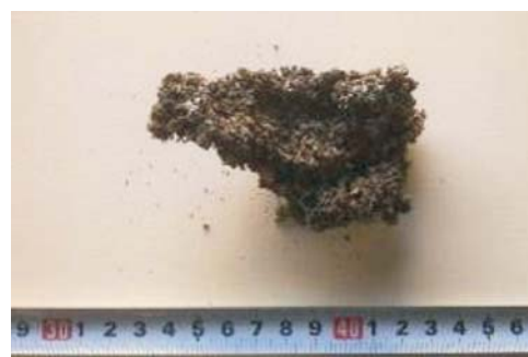
Figure 5. Photograph of an indicative agglomerate of olivine joined particles with cardoon ash
