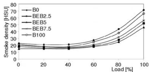
Figure 6. Variation of smoke emission with load for different fuels
