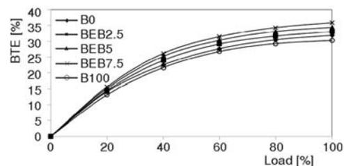
**Figure 2. Variation of BTE with load for different fuels**
