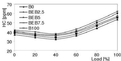
Figure 4. Variation of HC emission with load for different fuels
