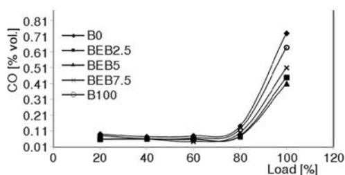
Figure 3. Variation of CO emission with load for different fuels
