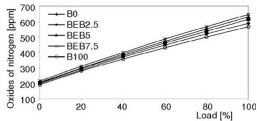
Figure 5. Variation of oxides of nitrogen emission with load for different fuels
