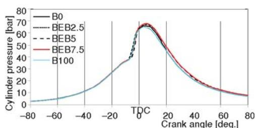
**Figure 7. Variation of cylinder pressure at full load for different fuels**
