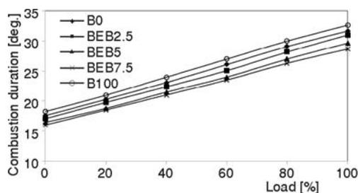
**Figure 8. Variation of combustion duration with load for different fuels**
