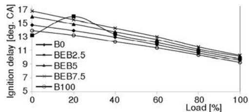
Figure 9. Variation of ignition delay with load for different fuels
