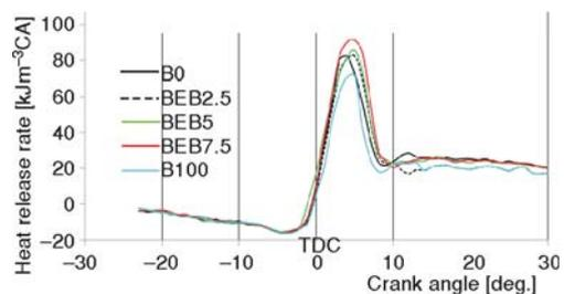
Figure 10. Variation of heat release rate at full load for different fuels
