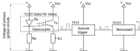
Figure 4. The principal scheme of the electronic block which produced the rectangular voltage signals synchronized with the sparks jumping on the spark plugs of engine
