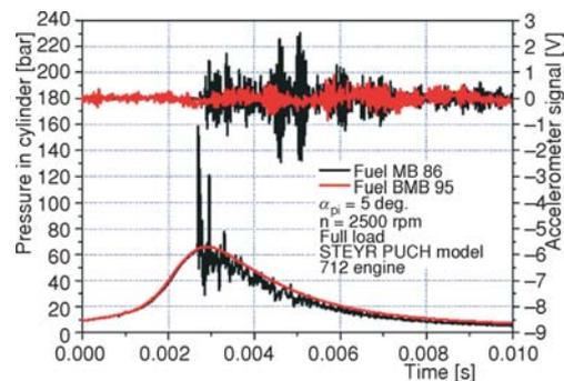
Figure 14. Comparative diagram of the change in pressure and accelerometer signal at 2500 rpm, maximum load and the pre-ignition static angle of 5 degrees with MB 86 and BMB 95 fuels (for color image see journal web site)
