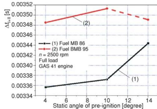
Figure 17. Distance between the moment of spark jump and reaching of the maximum pressure in the cylinder, in function of time, when using MB 86 and BMB 95 fuels
