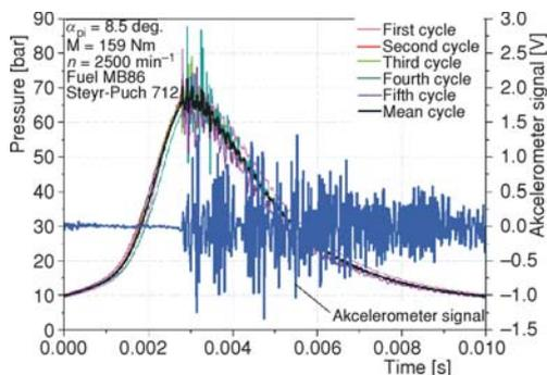
**Figure 6.** The flow of cylinder pressure and accelerometer mean signal of the accelerometer during five consecutive working cycles with detonative combustion in the STEYR-PUCH 712 engine at maximal load ( $\alpha_{pi} = 8.5$  deg., MB 86 fuel) (for color image see journal web site)
