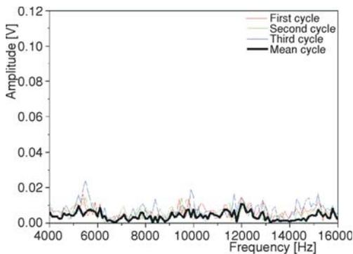
**Figure 10.** FFT analysis of accelerometer signals showed on fig. 8 (for color image see journal web site)
