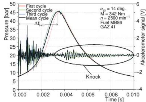
**Figure 9.** Flow of cylinder pressures and accelerometer signals during three working cycles of GAZ 41 engine with detonative combustion at maximal torque ( $\alpha_{pi} = 14$  deg., MB 86 fuel) (for color image see journal web site)
