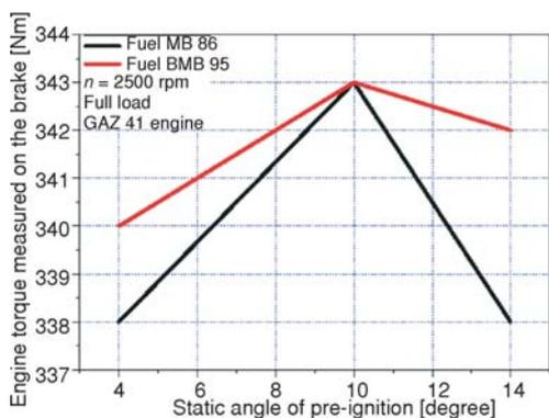
**Figure 15.** Dependence of the GAZ 41 engine maximal torque, measured on brake, on the set value of pre-ignition static angle for MB 86 and BMB 95 fuels
