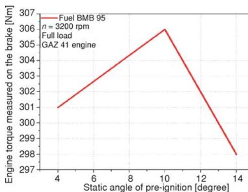
**Figure 16.** Dependence of the GAZ 41 engine maximal torque, measured on brake, on the set value of pre-ignition static angle for BMB 95 fuel at nominal regime (3200 rpm)
