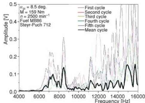
**Figure 7.** FFT analysis of accelerometer signals during five consecutive working cycles with detonative combustion in the STEYR-PUCH 712 engine at maximal load ( $\alpha_{pi} = 8.5$  deg., MB 86 fuel) (for color image see journal web site)
