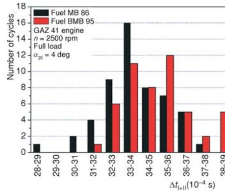
Figure 22. Cycle variations of the cumulative duration of the first and second theoretical combustion phase ( $\Delta t_{I+II}$ ) of the GAZ 41 engine for  $\alpha_{pi} = 4$  degree when using MB 86 and BMB 95 fuels
