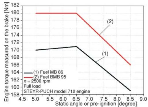
Figure 13. Change in maximum torque at 2500 rpm in the function of pre-ignition static angle for two different types of fuel (MB 86 and BMB 95)
