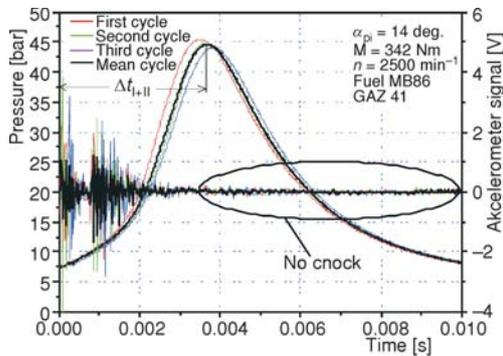
**Figure 8.** Flow of cylinder pressures and accelerometer signals during three working cycles of GAZ 41 engine without noticeable detonative combustion at maximal torque ( $\alpha_{pi} = 14$  deg., BMB 95 fuel) (for color image see journal web site)
