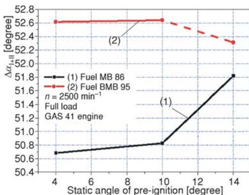
Figure 18. Distance between moments of spark jump and maximum pressure in the cylinder, estimated in the function of the crankshaft angle, when using MB 86 and BMB 95 fuels
