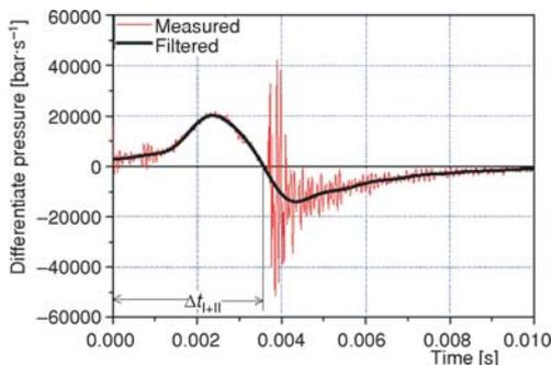
**Figure 12. Typical diagram of the change of pressure differential (GAZ 41 engine)**
