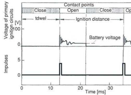
Figure 3. The voltage change of the primary of the ignition circuit of the distributor and the rectangular impulses generated in the electronic block
