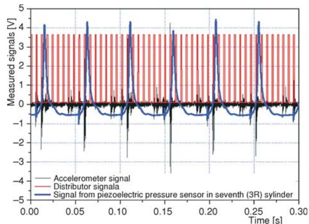
Figure 5. The typical diagram of the measured signals on the GAZ 41 engine recorded
