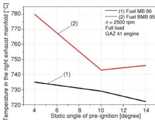
Figure 21. Dependence of exhaust gases temperature in the right exhaust manifold on pre-ignition static angle and type of used petrol at maximal torque regime
