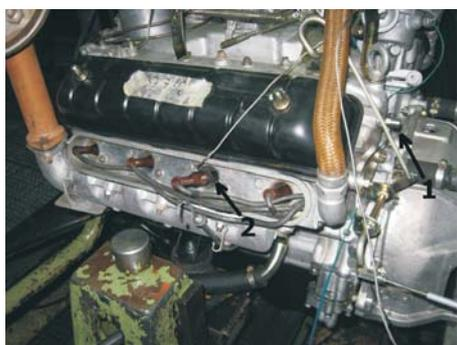
**Figure 2. The arrows show the locations of the vibration sensors – the accelerometer (Bruel & Kjer type 4321) and the spark plugs with an integrated piezoelectric pressure sensor (Kistler) on the GAZ 41 engine**
