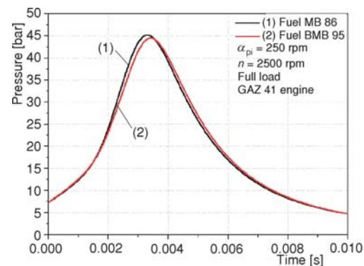
Figure 19. Mean cycles of pressure change in the same test conditions ( $\alpha_{pi} = 4$  deg.,  $n = 2500$  rpm, full load), but with different types of fuel (MB 86 and BMB 95)
