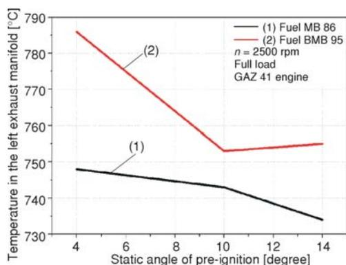
Figure 20. Dependence of exhaust gases temperature in the left exhaust manifold, on pre-ignition static angle and the type of the used petrol at maximal torque regime
