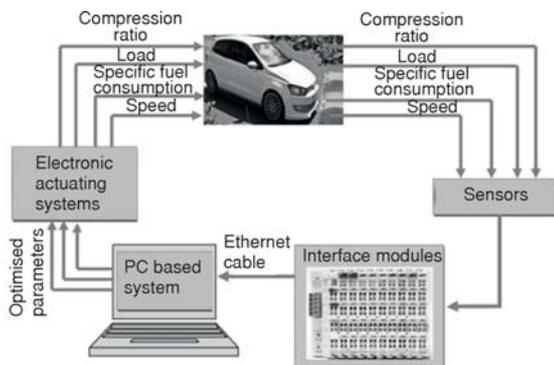
Figure 1. Intelligence based diesel engine performance control system
