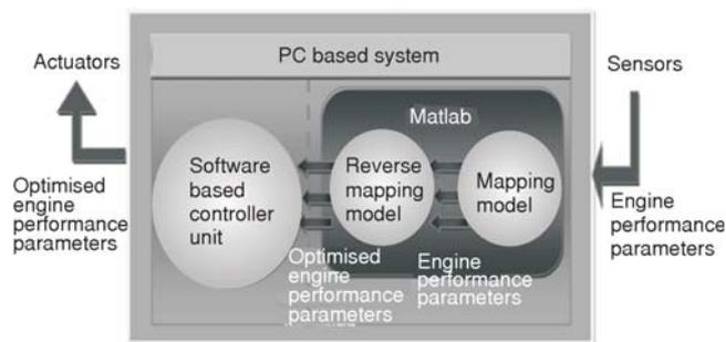
Figure 2. Parameter mapping and control system framework
