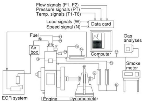
**Figure 3. Experimental set-up of variable compression diesel engine**
