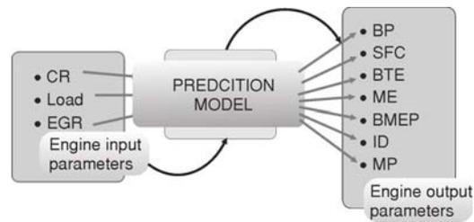
**Figure 11. Prediction model using SVM for various engine performance parameters**
