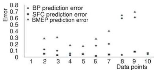
Figure 16. SVM prediction error values for BP, SFC, and BMEP
