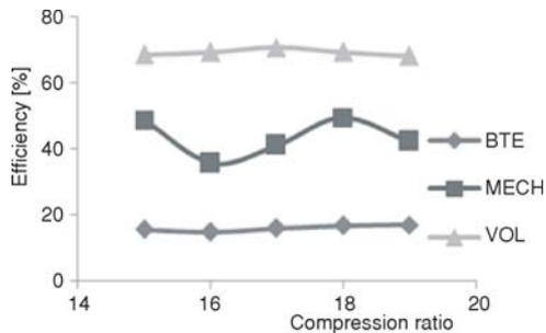
Figure 4. Effect of CR on BTE, ME, and VE at 25% load
