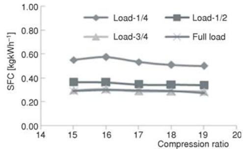
Figure 5. Effect of CR on SFC at different loads
