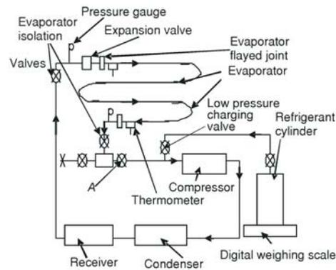
**Figure 1. Schematic equipment set-up for charging the system**
