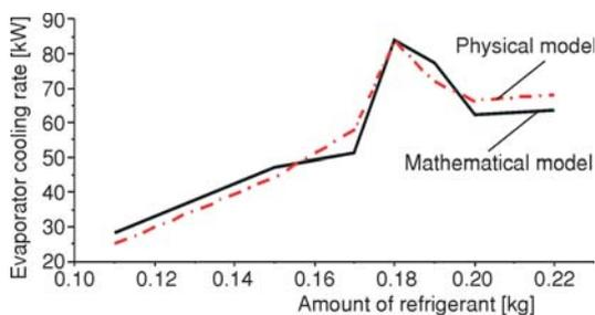
Figure 4. Physical and mathematical evaporator cooling rate curve of area 0.06285 m<sup>2</sup> per meter
