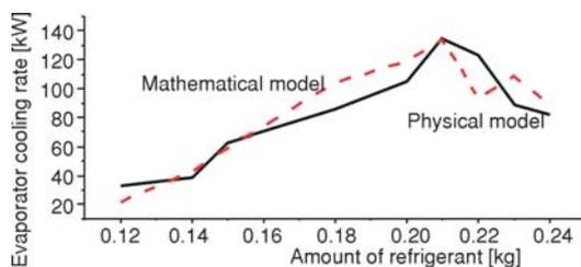
Figure 9. Physical and mathematical evaporator cooling curve of area 0.08180 m<sup>2</sup> per meter
