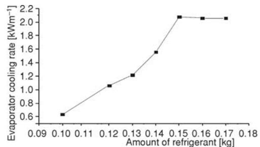
**Figure 8.** Evaporator cooling rate curve of area 0.04712 m<sup>2</sup> per unit length
