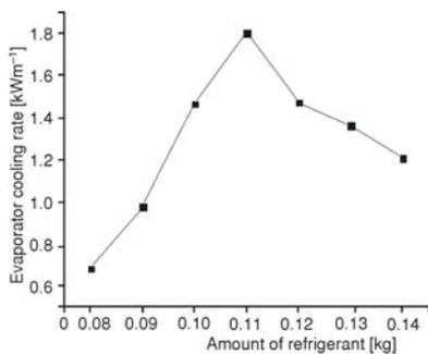
**Figure 5.** Evaporator cooling rate curve of an evaporator of area 0.015716 m<sup>2</sup> per meter
