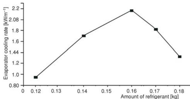
**Figure 6.** Evaporator cooling rate curve of area 0.06283 m<sup>2</sup> per unit length
