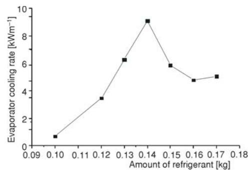
**Figure 7.** Evaporator cooling rate curve of an evaporator of area 0.03142 m<sup>2</sup>
