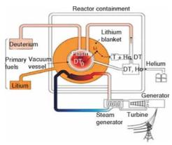
Figure 6. Fusion power plant
