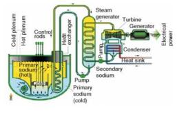
Figure 5. FBR with closed fuel cycle
