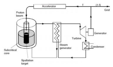
Figure 7. Accelerator driven system - ADS
