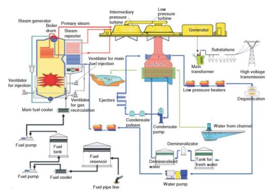
Figure 8. Thermal power plant
