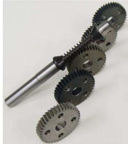
**Figure 3. Worm and gears of different material variants**
