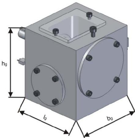
Figure 8. Dimensions of test gear drive
