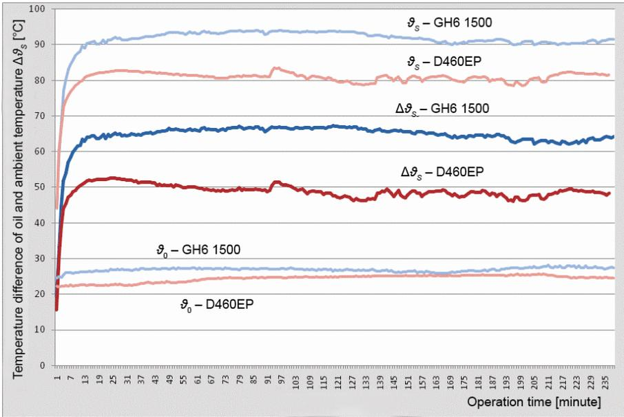
Figure 4. Temperature difference of oil and ambient air temperature for worm and gear set and  $T_2 = 24 \text{ Nm}$
