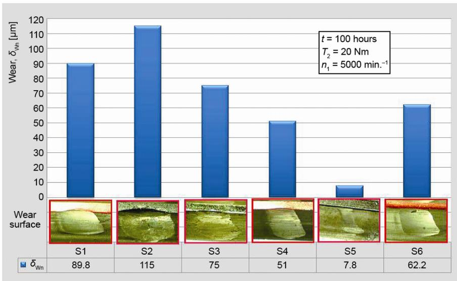
Figure 12. Wear rate  $\delta_{wn}$  for all experiments with different material variants [10]
