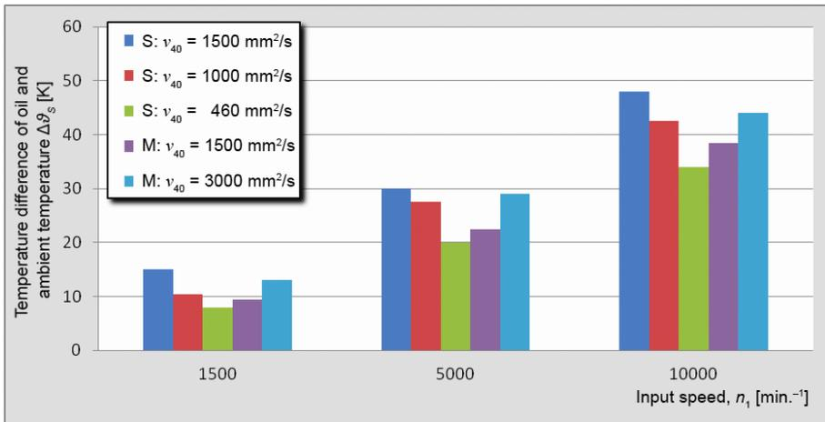
Figure 6. Temperature difference between oil and ambient air temperature for synthetic and mineral oil (S and M) depending on viscosity and input speed  $n_1$
