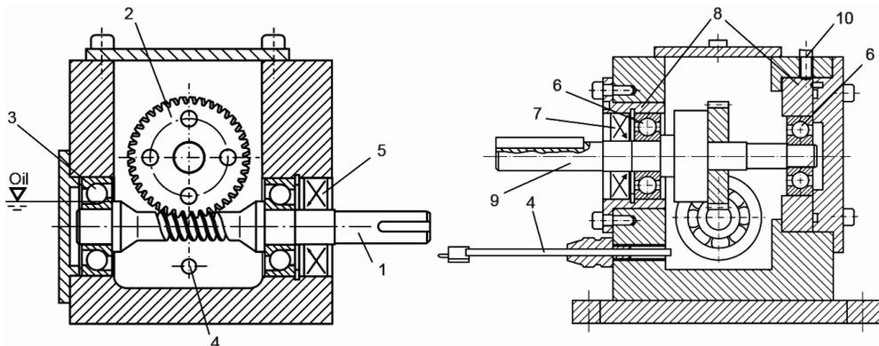
**Figure 2. Sectional drawings of test transmission**
