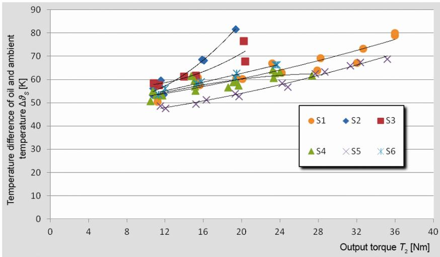
Figure 9. Comparison of measured temperature difference between oil and ambient air of worm and gear set with gear made of sintered steel with different additional treatments for  $n_1 = 5000 \text{ min.}^{-1}$
