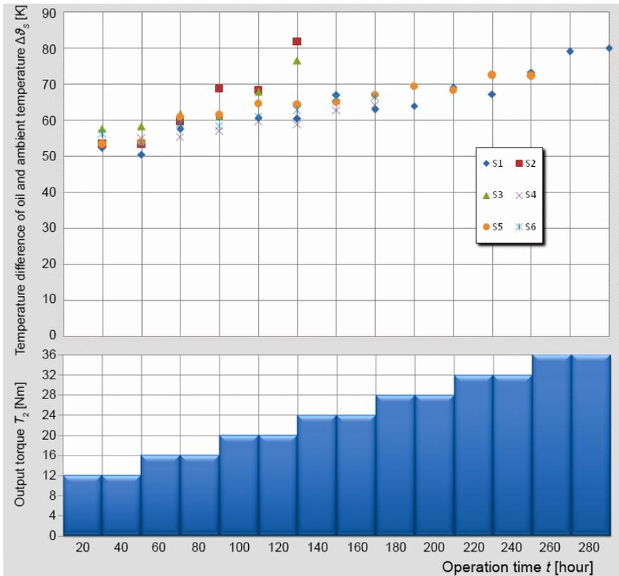
Figure 10. Temperature difference between oil and ambient air as function of operational time for different material variants and  $n_1 = 5000 \text{ min.}^{-1}$
