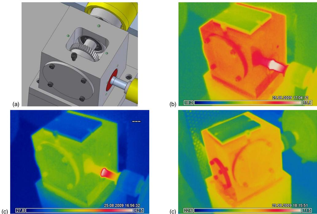
Figure 7. 3-D view and thermal image of the test gear drive [°C]
