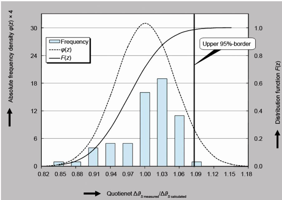
Figure 11. Distribution for determination of minimal temperature safety coefficient
