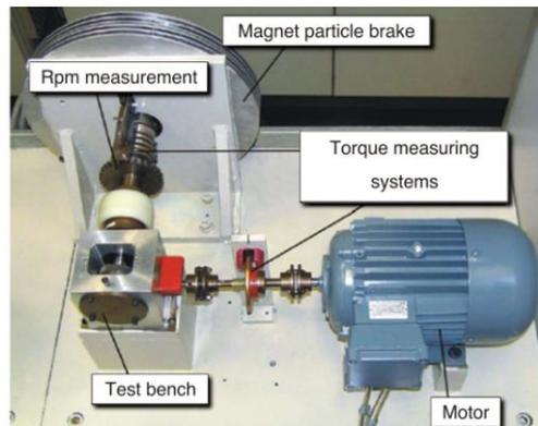
**Figure 1. Gear test rig**
