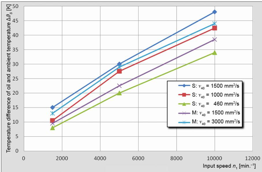
Figure 5. Temperature difference between oil and ambient air temperature for synthetic and mineral oil (S and M) depending on viscosity and input speed  $n_1$
