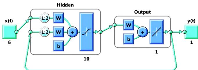
Figure 6. NARX neural network used for CO<sub>2</sub> emission estimation
