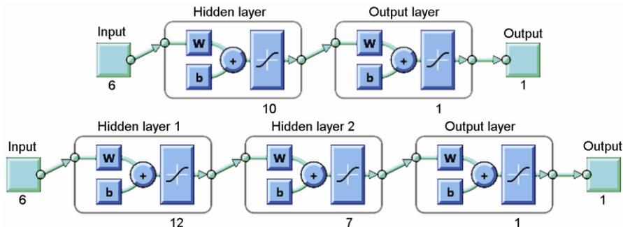
**Figure 4.** Neural networks with one and two hidden layers used for CO<sub>2</sub> emission estimation
