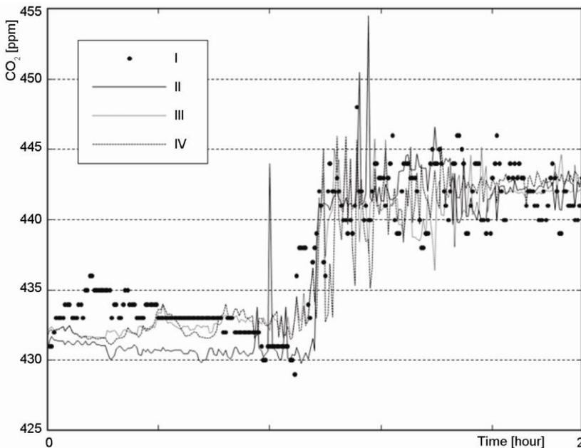
**Figure 7. Experimental verification of accuracy of trained neural networks and ANFIS model: I – measured data, II – estimation of ANN with one hidden layer, III – estimation of ANN with two hidden layers, and IV – estimation of ANFIS**
