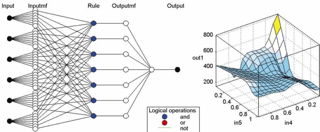
Figure 5. (a) ANFIS structure used for CO<sub>2</sub> emission estimation and (b) fuzzy model output surface
