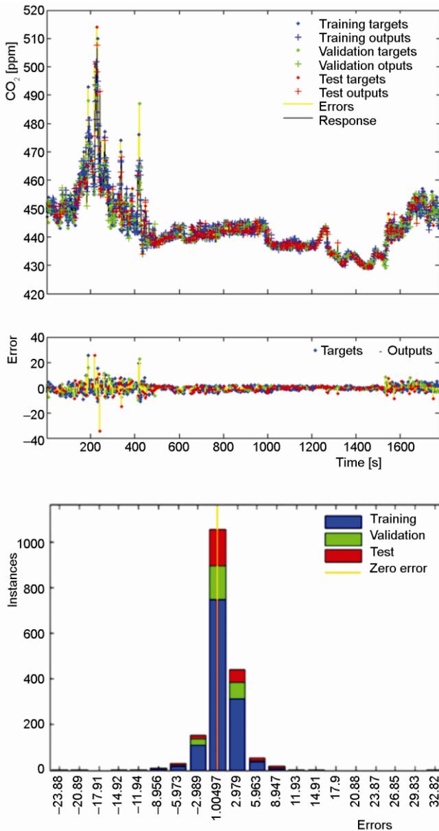
**Figure 8. Experimental verification of accuracy of trained NARX neural network, error diagram, and error distribution**
