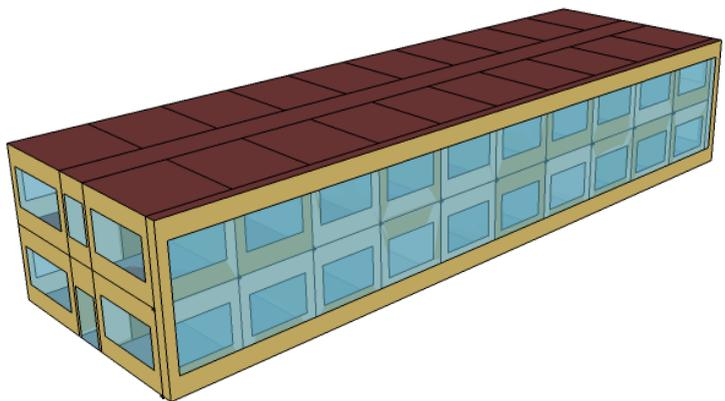
Figure 1. Isometric view of the office building with double skin façade
