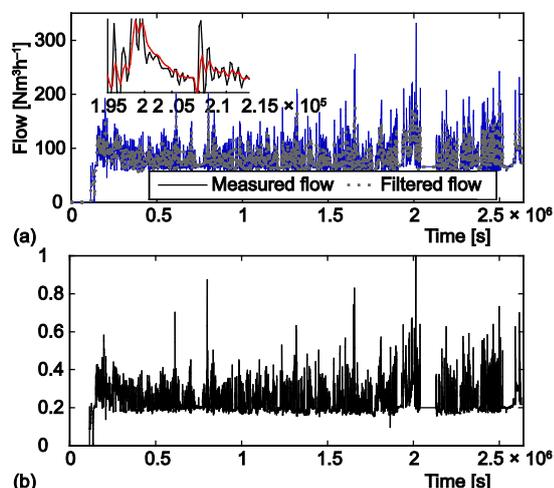
**Figure 2. Effects of data pre-processing on gas flow signal of zone 4; (a) low pass filter, (b) normalization (for color image see journal web-site)**
