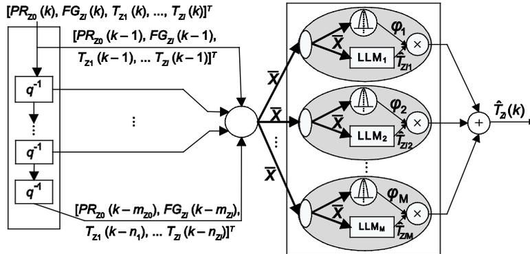
Figure 5. Typical structure of the one-step neuro-fuzzy predictive model; combination of the static LLNF network and TDL filters
