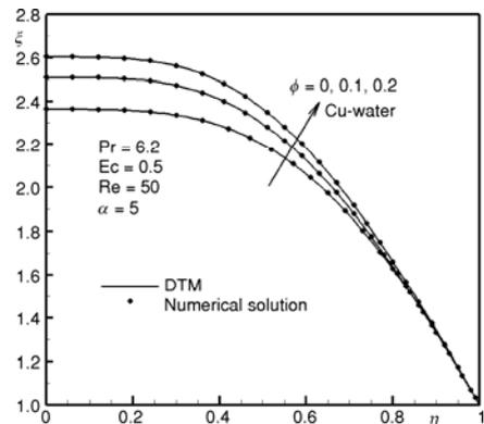
Figure 6. Variation of  $\xi(\eta)$  with different values of solid volume fraction for water-Cu nanofluid when  $Re = 50$ ,  $Ec = 0.5$ , and  $\alpha = 5$
