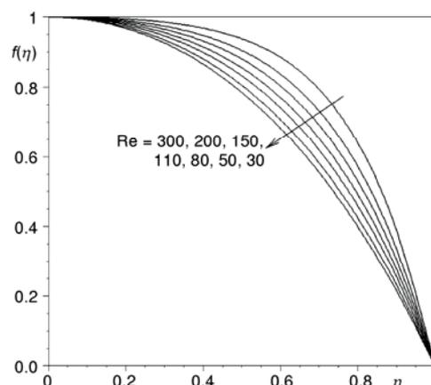
Figure 10. The effect of Reynolds number on  $f(\eta)$  for water- $TiO_2$  nanofluid when  $\alpha = -3$  and  $\phi = 0.1$
