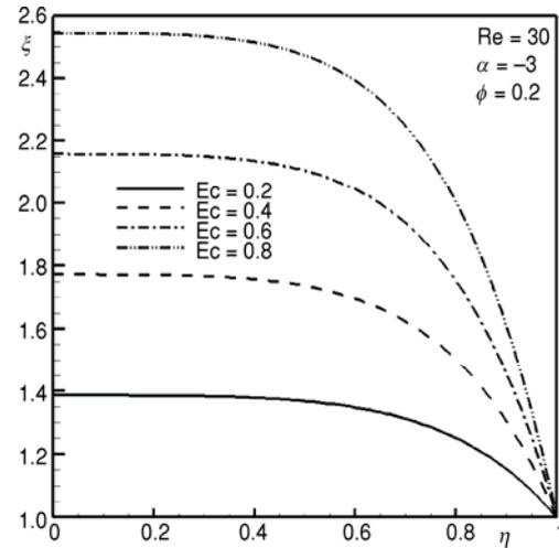
Figure 12. The effect of Eckert number  $Ec$  on  $\xi(\eta)$  for water-Cu nanofluid when  $\alpha = -3$ ,  $\phi = 0.2$ , and  $Re = 30$
