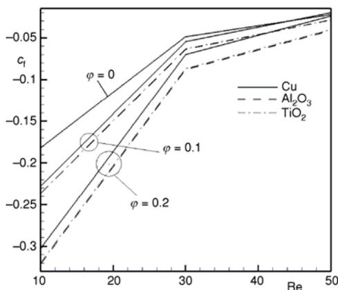
Figure 13. The variation of skin friction coefficient with Reynolds number in three types of nanoparticles for different solid volume fraction
