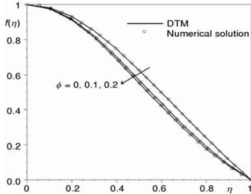
Figure 2. Variation of  $f(\eta)$  with different values of solid volume fraction for water-Cu nanofluid when  $Re = 50$  and  $\alpha = 5$
