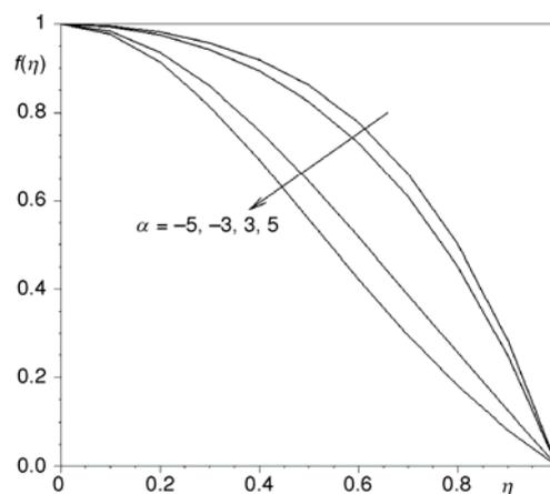
Figure 8. The effect of angle  $\alpha$  on  $f(\eta)$  for water- $Al_2O_3$  nanofluid when  $\phi = 0.2$ , and  $Re = 50$
