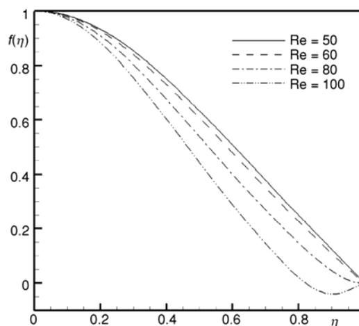
**Figure 15. The effect of Reynolds number  $Re$  on  $f(\eta)$  for water-TiO<sub>2</sub> nanofluid when:  $\varphi = 0.1$  and  $\alpha = 5$  in a divergent channel**
