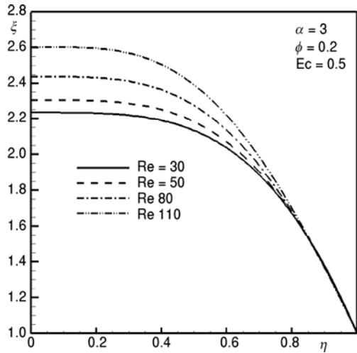
Figure 11. The effect of Reynolds number  $Re$  on  $\varphi(\eta)$  for water-TiO<sub>2</sub> nanofluid when  $\alpha = 3$ ,  $Ec = 0.5$  and  $\phi = 0.2$
