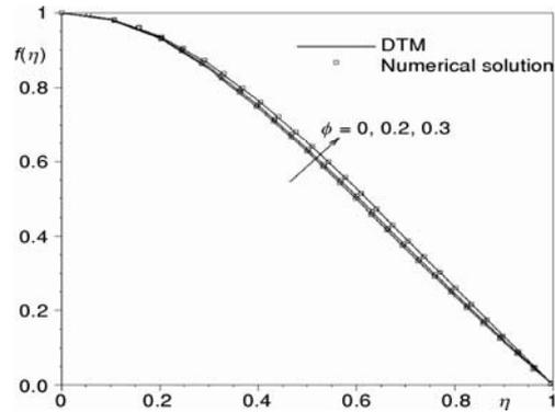
Figure 4. Variation of  $f(\eta)$  with different values of solid volume fraction for water- $TiO_2$  nanofluid when  $Re = 50$  and  $\alpha = 5$
