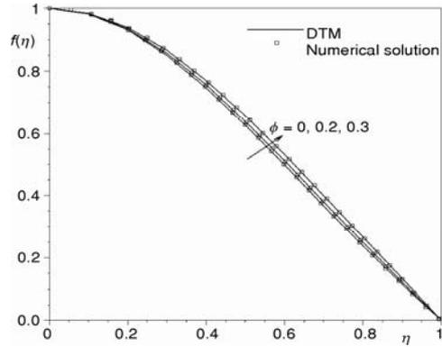
Figure 3. Variation of  $f(\eta)$  with different values of solid volume fraction for water- $Al_2O_3$  nanofluid when  $Re = 50$  and  $\alpha = 5$
