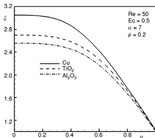
Figure 7. Variation of  $\xi(\eta)$  for three types of nanoparticles when  $Re = 50$ ,  $\alpha = 7$ ,  $Ec = 0.5$ , and  $\phi = 0.2$
