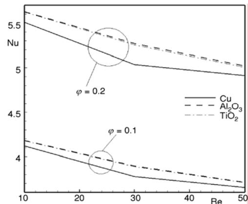
Figure 14. The variation of Nusselt number with Reynolds number in three types of nanoparticles for different solid volume fraction
