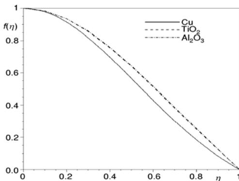
Figure 5. Variation of  $f(\eta)$  for three types of nanoparticles when  $Re = 80$ ,  $\alpha = 3$ , and  $\phi = 0.2$
