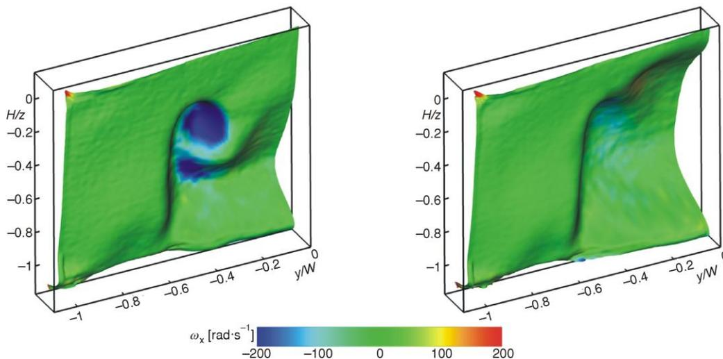
**Figure 3.** Longitudinal vorticity field in a transverse plane behind the Ahmed model ( $x/L = 0.4$ ) from SPIV measurements, without (left) and with control device (right). The depth of this vorticity field corresponds to the longitudinal velocity component (color image see on our web site)
