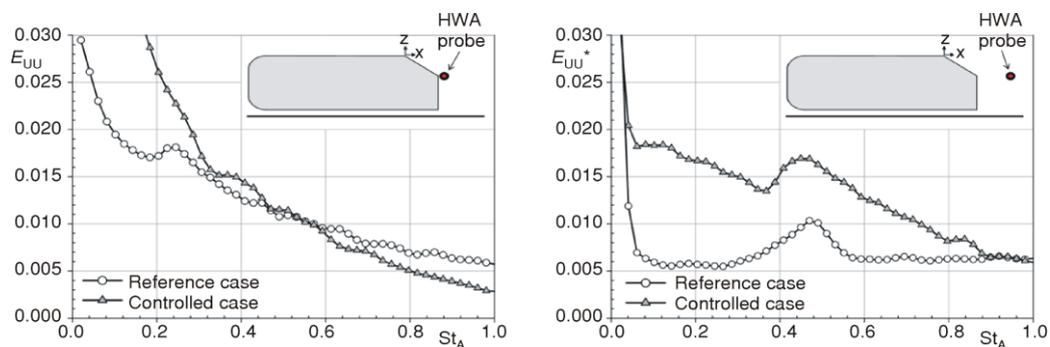
**Figure 7.** Power spectral densities in two different points downstream the model, at  $x/L = 0.2$  (left) and  $0.4$  (right); ( $E_{uu}$  is the energy spectrum of the streamwise velocity component, normalized by its variance)
