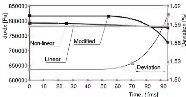
Figure 1. Comparison of  $dp/dx$  models and modified model's standard deviation [%]
