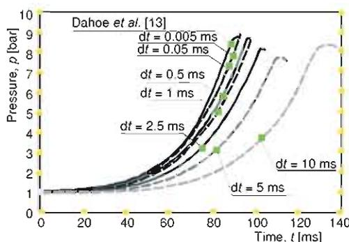
Figure 2. Results of numerical integration of the expression (1) for different magnitude of time steps from 0.005 to 10 ms [13]
