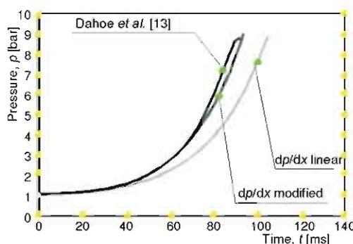
Figure 3. Comparison of the experiment with modified pressure raise function model, and linear pressure raise function model [13]
