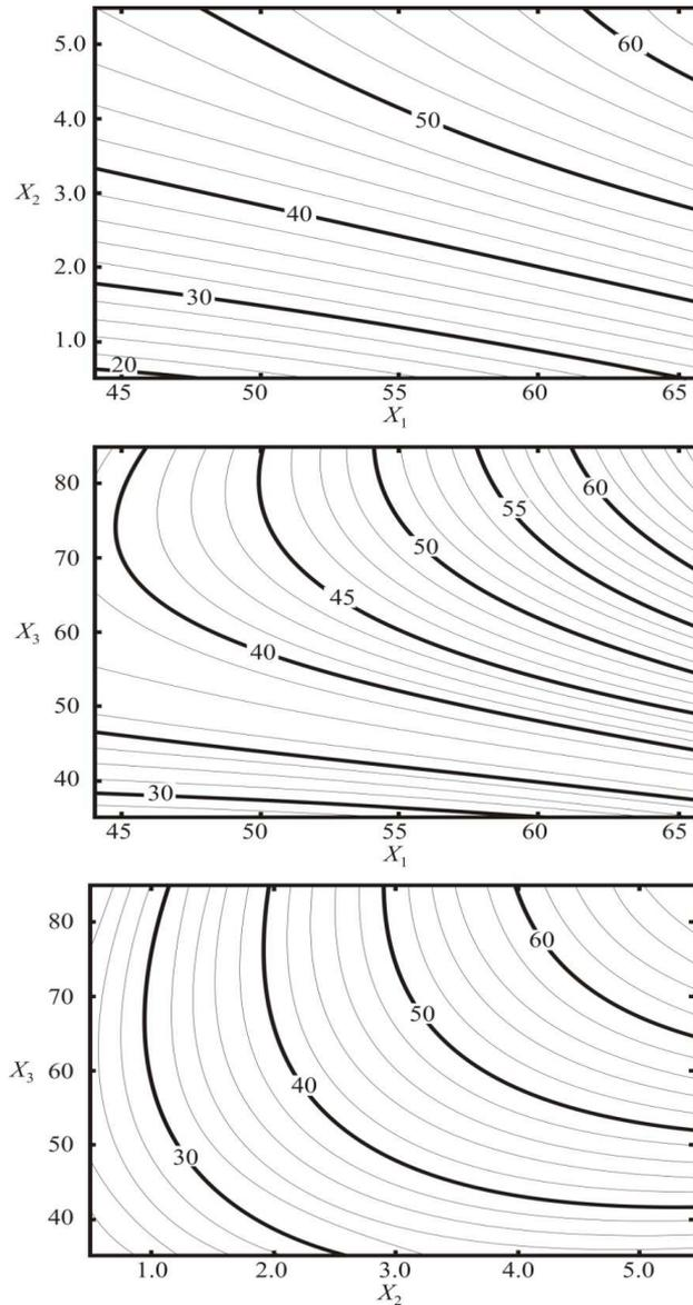
**Figure 1. Contour plots for  $DM$  as function of temperature ( $x_1$ ), time ( $x_2$ ) and sugar concentration ( $x_3$ )**
