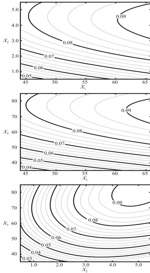
**Figure 3. Contour plots for  $S_g$  as function of temperature ( $x_1$ ), time ( $x_2$ ) and sugar concentration ( $x_3$ )**
