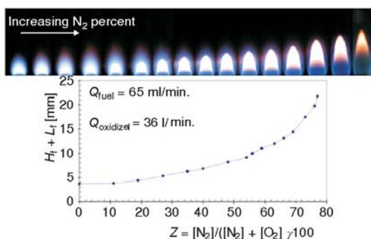
Figure 6. Effects of diluting oxygen with  $N_2$  along with natural gas fuel; each point on the figure matches with one of the flames from left to right, respectively
