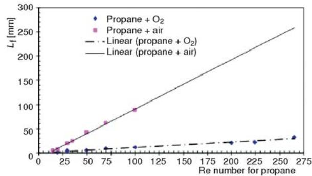
Figure 3. Propane flame length variations with increasing fuel stream velocity for air and oxygen
