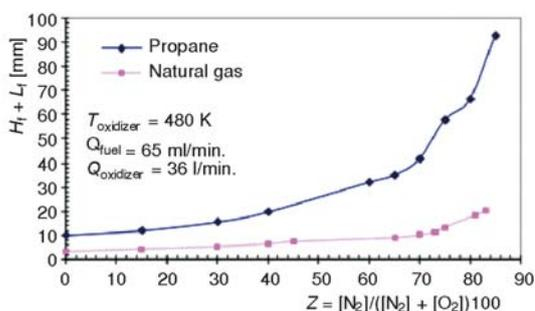
Figure 13. Effect of changing fuel type on preheating and diluting oxygen oxidizer with nitrogen
