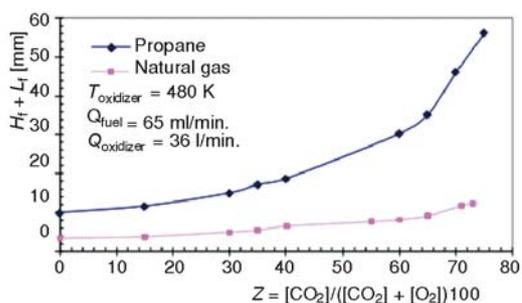
Figure 12. Effect of changing fuel type on preheating and diluting oxygen oxidizer with carbon dioxide
