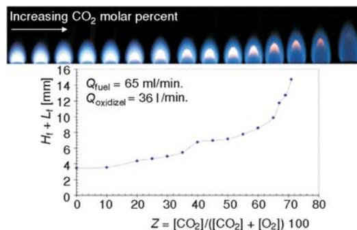
Figure 7. Effects of diluting oxygen with CO<sub>2</sub> along with natural gas fuel each points on the figure matches with one of the flames from left to right, respectively
