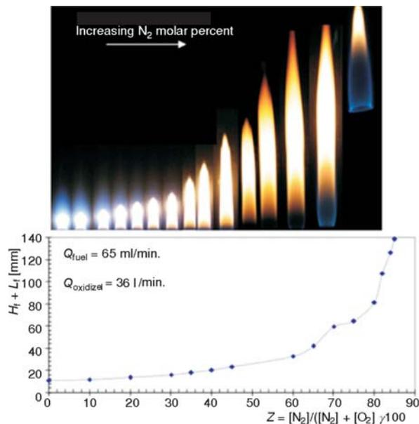
Figure 4. Effects of diluting oxygen with N<sub>2</sub> along with propane fuel; each point on the figure matches with one of the flames from left to right, respectively
