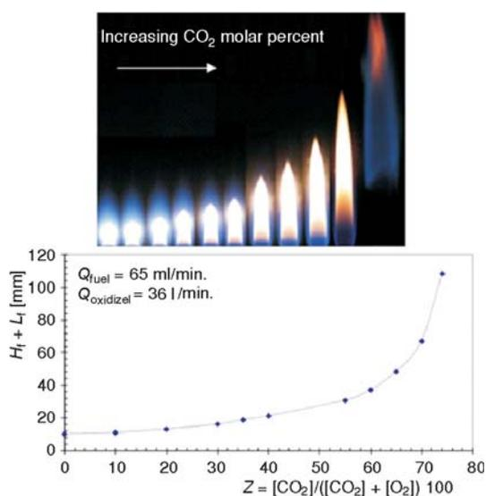
Figure 5. Effects of diluting oxygen with  $CO_2$  along with propane fuel; each point on the figure matches with one of the flames from left to right, respectively
