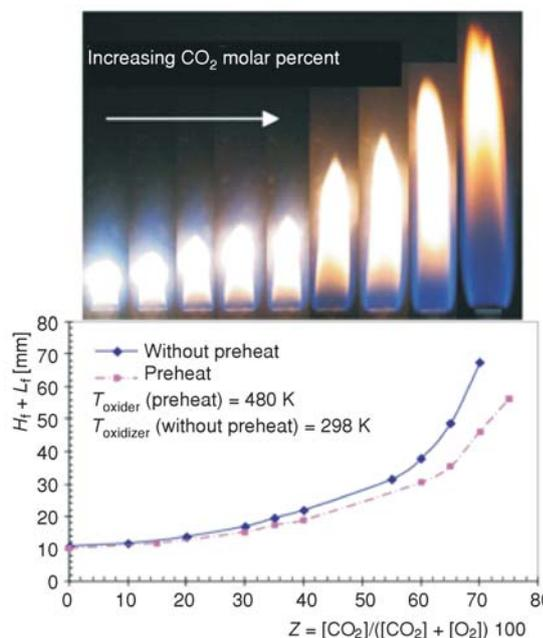
Figure 8. Comparing flame lift-off and height sum with dilution percent in diluting oxygen with carbon dioxide and with propane fuel in oxidant preheating and non-preheating states
