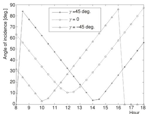
Figure 9. Angle of incidence of solar radiation on the input aperture vs. hour
