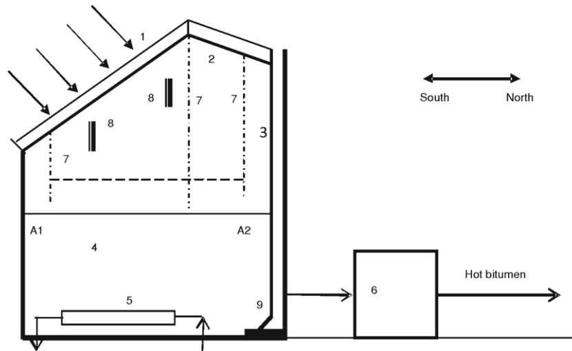
**Figure 5. Diagram of the classical and solar installation for bitumen preheating)**
