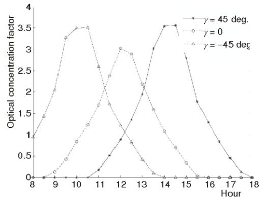
Figure 11. Optical concentration efficiency vs. hour
