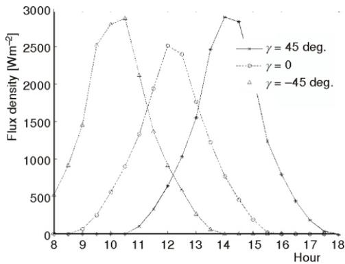
Figure 10. Radiant flux density on the photovoltaic cell vs. hour
