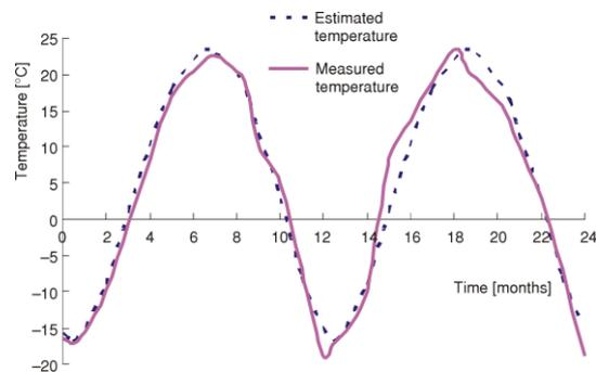
Figure 2. Air temperature in Fengman dam location vs. seasons from 1980 to 1981
