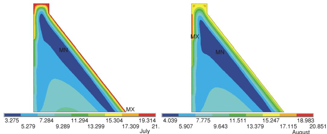
Figure 5. Temperature distribution of transverse section of the Fengman dam in July and August (unit: °C) (color image see on our web site)
