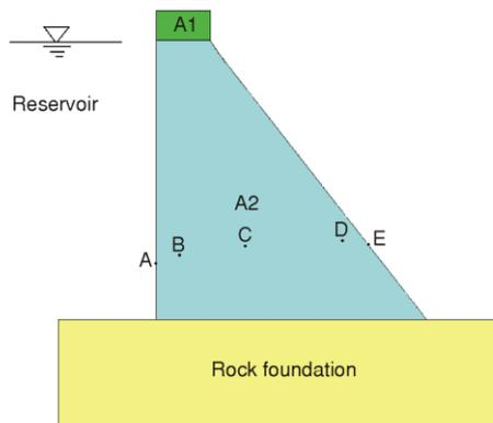
Figure 1. Basic model of dam and rock foundation for computing thermal transfer
