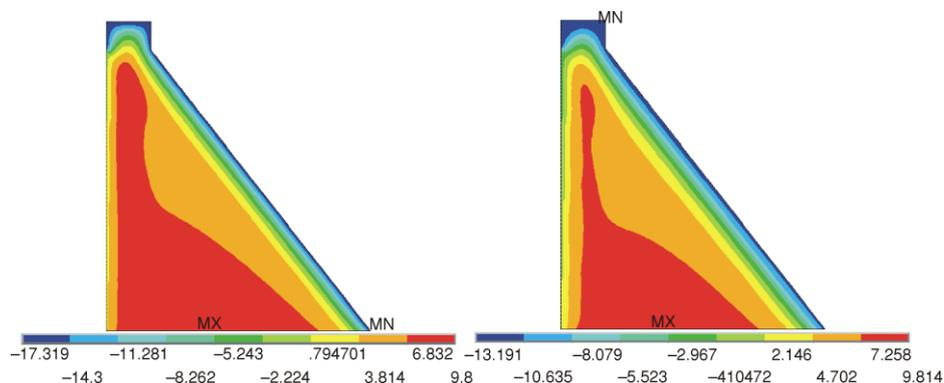
**Figure 4. Temperature distribution of transverse section of the Fengman dam in January and February (unit:  $^{\circ}\text{C}$ ) (color image see on our web site)**
