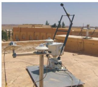
Figure 2. Sun-Tracker station installed at applied research unit on renewable energies
