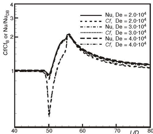
Figure 5. Skin friction and Nusselt number distributions along the outer wall (y-z plane)
