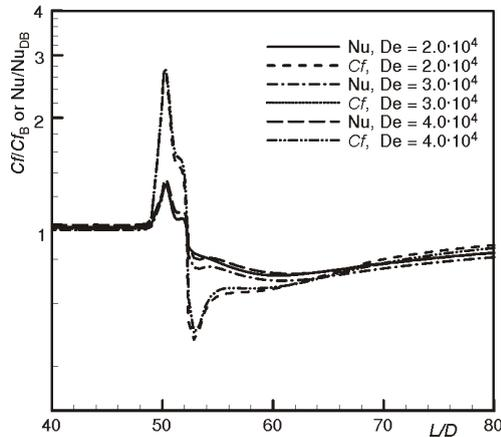
Figure 4. Skin friction and Nusselt number distributions along the inner wall (y-z plane)
