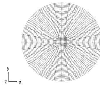
Figure 2. Mesh at a cross-section of the U-tube (x-y plane)
