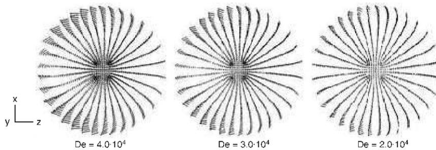
Figure 7. Velocity vectors at the mid-section of the curved tube (x-z plane)
