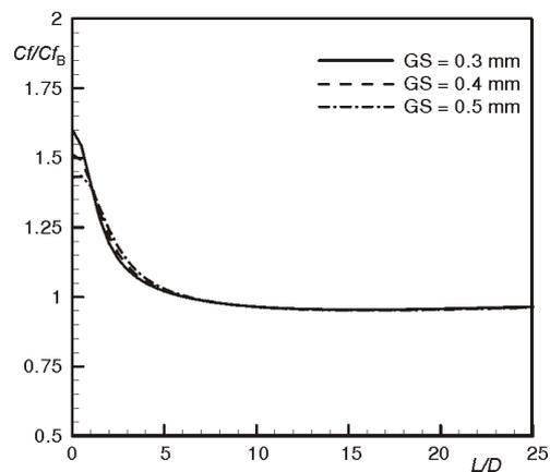
Figure 3. Upstream skin friction distribution for different grid spacing (GS)
