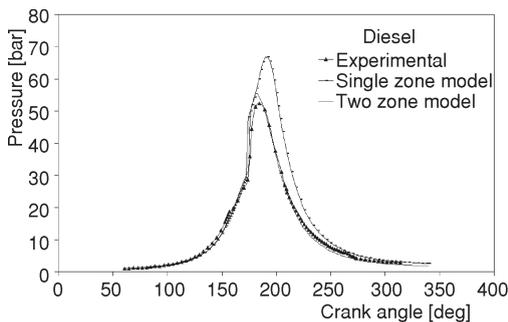
Figure 3. Comparison of cylinder pressures of diesel
