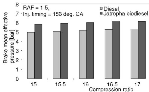
Figure 13. Effect of compression ratio on brake mean effective pressure
