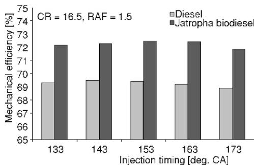
**Figure 6.** Effect of injection timing on mechanical efficiency
