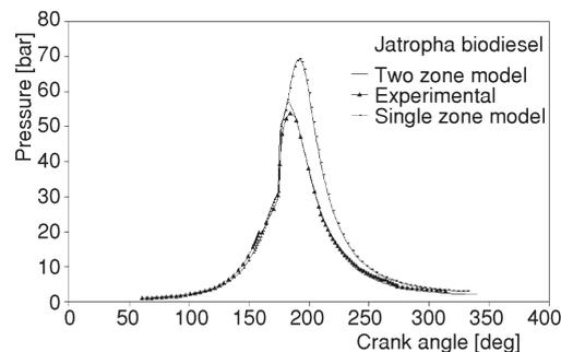
Figure 4. Comparison of cylinder pressures of jatropha biodiesel
