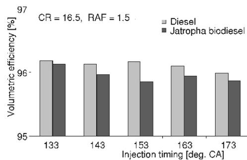
**Figure 7.** Effect of injection timing on volumetric efficiency
