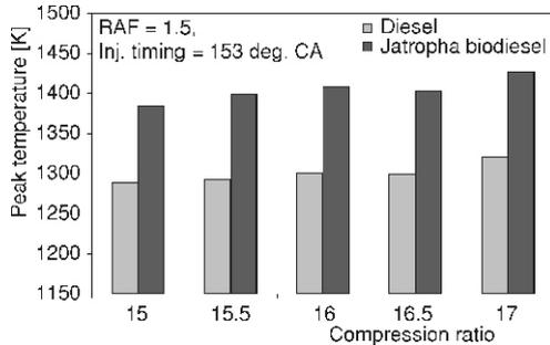
**Figure 14. Effect of compression ratio on peak temperature**
