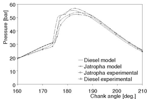
**Figure 17. Comparison of calculated and experimental cylinder pressure**
