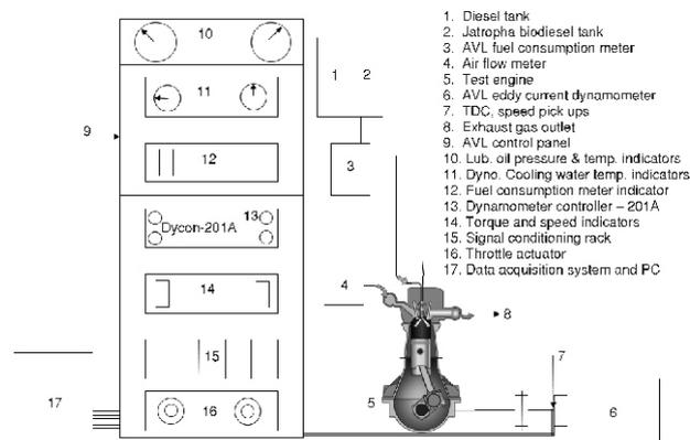
**Figure 2. Schematic diagram of the experimental setup**
