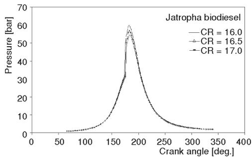
Figure 10. Effect of compression ratio on cylinder pressure
