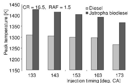
**Figure 9.** Effect of injection timing on peak temperature
