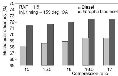
Figure 12. Effect of compression ratio on mechanical efficiency
