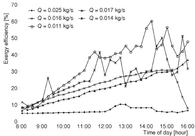
**Figure 8. Exergy efficiency during winter per different mass flow rates in the day times**
