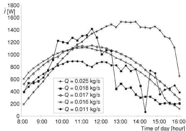
Figure 7. Irreversibility during winter for different mass flow rates *vs.* day time
