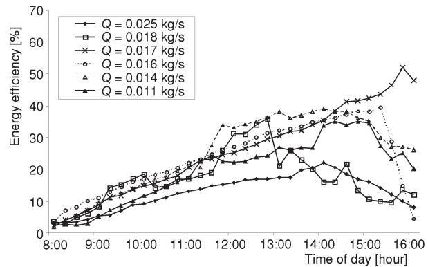
Figure 6. Energy efficiency during winter as a function of day time at different flow rate
