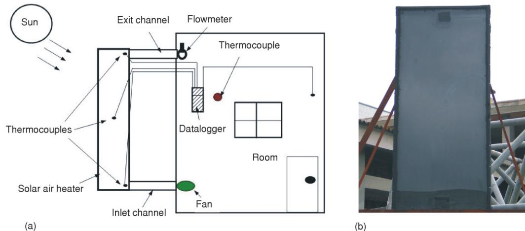
**Figure 2.** A schematic of test setup and photo of the collector [23]
