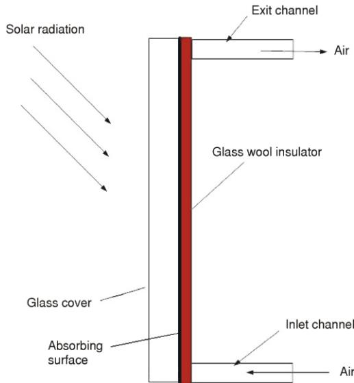
**Figure 1.** A schematic of the designed collector [23]
