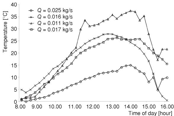
**Figure 4. Average air temperature variation in winter at different flow rates**
