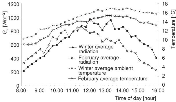
**Figure 3. Average radiation intensity and ambient temperature in winter**
