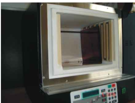
Figure 2. Placing the radiant panels inside the working area of the furnace
