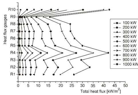
Figure 11. Total heat flux changes with HRR in Test 7
