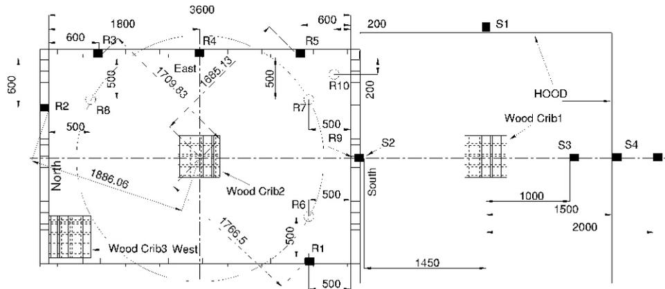
Figure 1. Location of wood cribs and heat flux gauges
