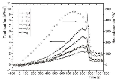
Figure 2. Time history of HRR and total heat flux in Test1
