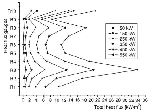
**Figure 15. Total heat flux changes with HRR in Test11**
