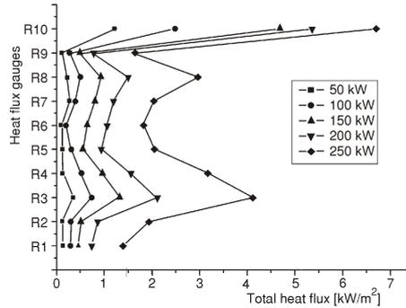
same shape for almost all gauges in this test as in Test9. But R2 changed back to Test8 which was lower than both R4 but higher than R5. R10 was lower than R3 at the end of test. Figure 15 shows the results from Test11. The most outstanding characteristics of Test11 is the total heat flux to the floor reached to a very high level and were close to heat flux to the wall. The peak heat flux of R3 was not as high as R3 in Test10 even the HRR reached 900 kW in Test11.
