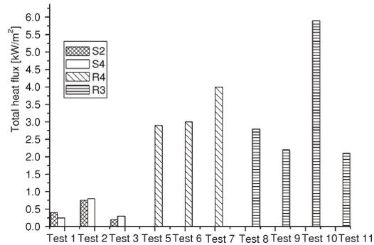
**Figure 18. S2, S4, R3, and R4 value at HRR = 500 kW**
