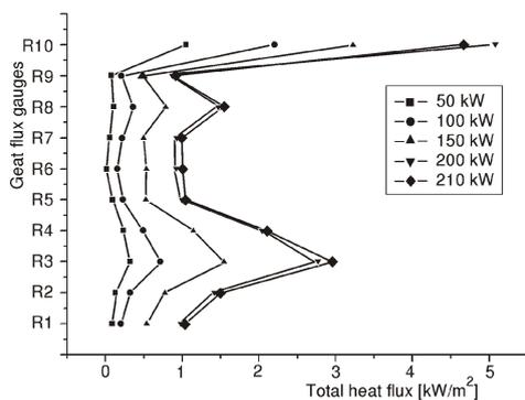
Figure 12. Total heat flux changes with HRR in Test8
