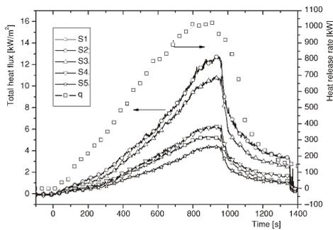
Figure 4. Time history of HRR and total heat flux in Test2
