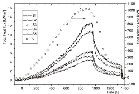
Figure 6. Time history of HRR and total heat flux in Test3
