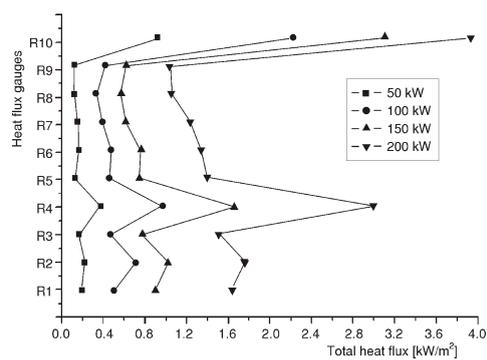
**Figure 9. Total heat flux changes with HRR in Test 5**
