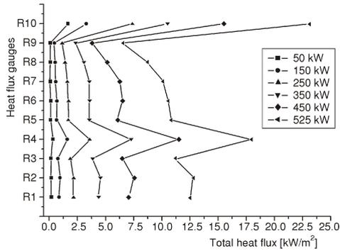
Figure 10. Total heat flux changes with HRR in Test 6
