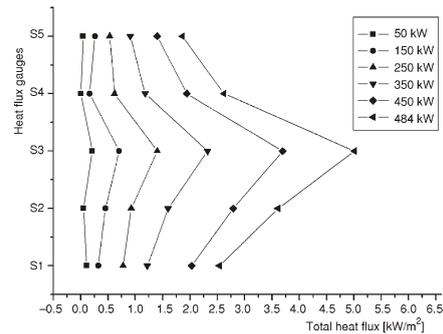
Figure 3. Total heat flux changes with HRR in Test1
