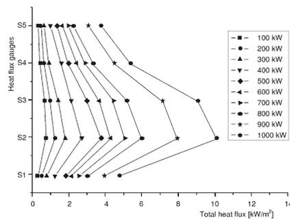
Figure 5. Total heat flux changes with HRR in Test2
