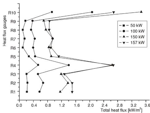
**Figure 8. Total heat flux changes with HRR in Test4**
