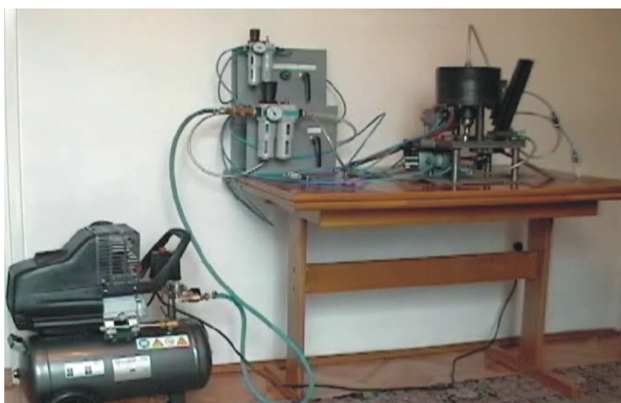
Figure 4. Laboratory pneumatic press for pellet manufacturing [15]
