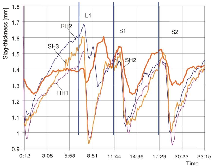
Figure 6. Slag thickness / Soot blowing (L – light, S – strong)
