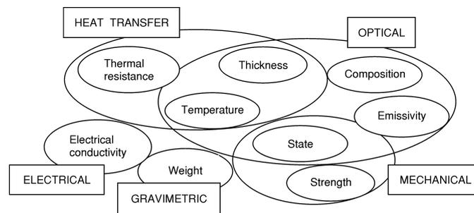
**Figure 2. Physical properties / Measurement methods**
