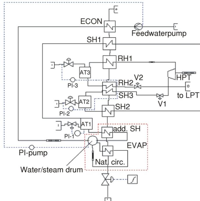
**Figure 4. Flow sheet of the overall plant model**
