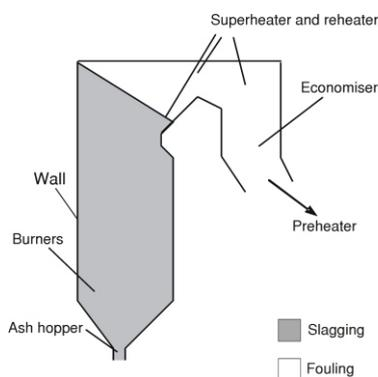
**Figure 1. S&F in a pulverized fuel boiler**
