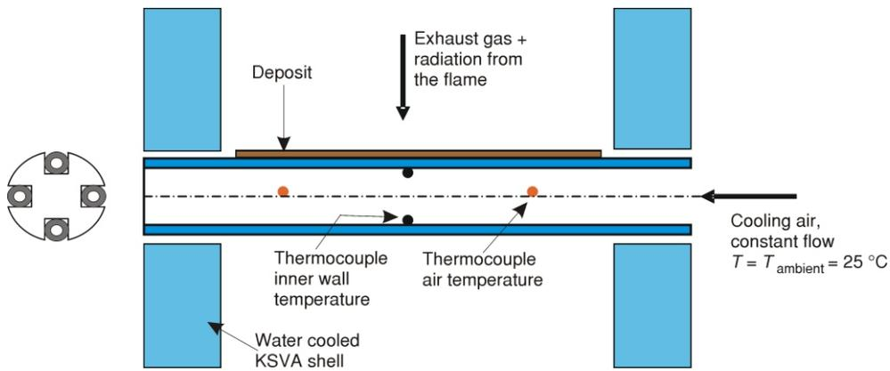
Figure 5. Probe and inner rod with four thermocouple housings
