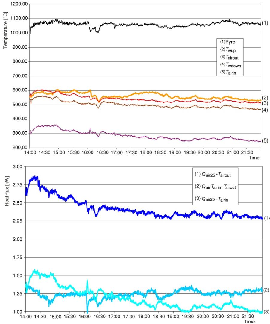
**Figure 7. Experimental results: temperatures and heat flux**
