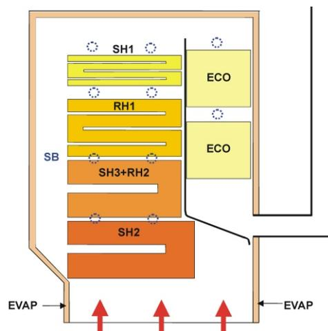
Figure 3. Structure of the boiler
